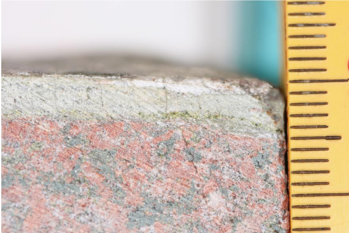
Figure 4-2. Photographed cross-section of core with visible fracture minerals.
