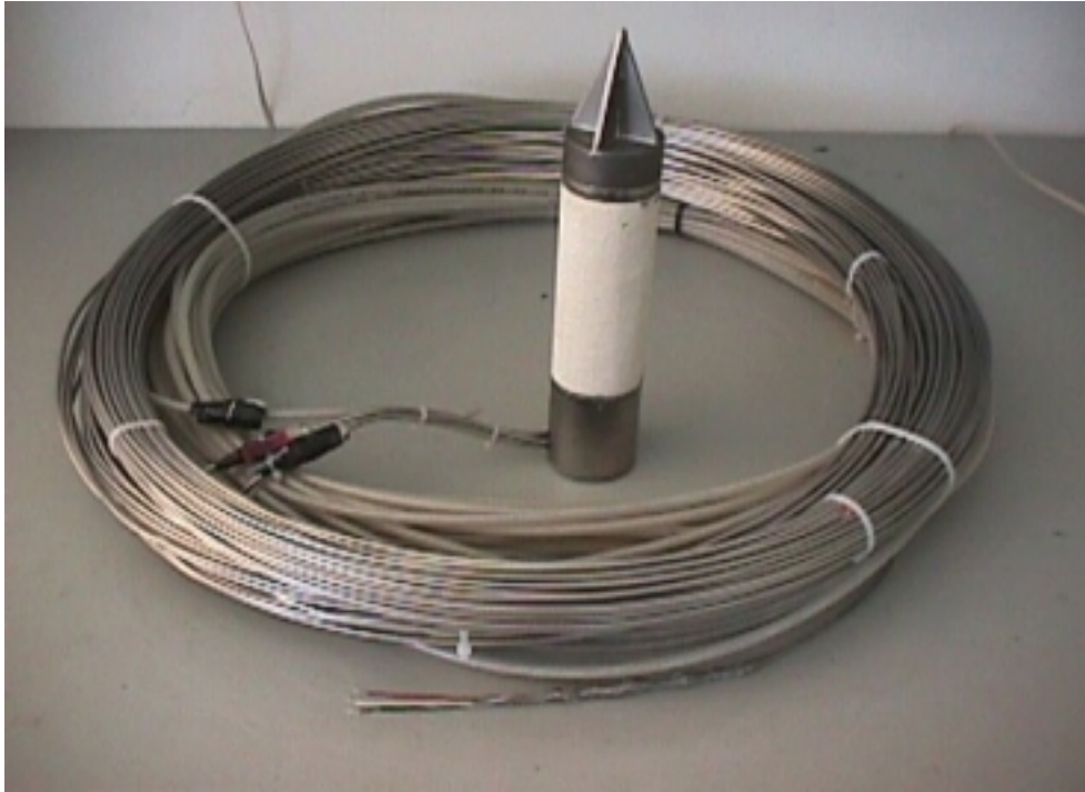
Figure 7-15. View of a dynamic pore pressure sensor (DPP).
