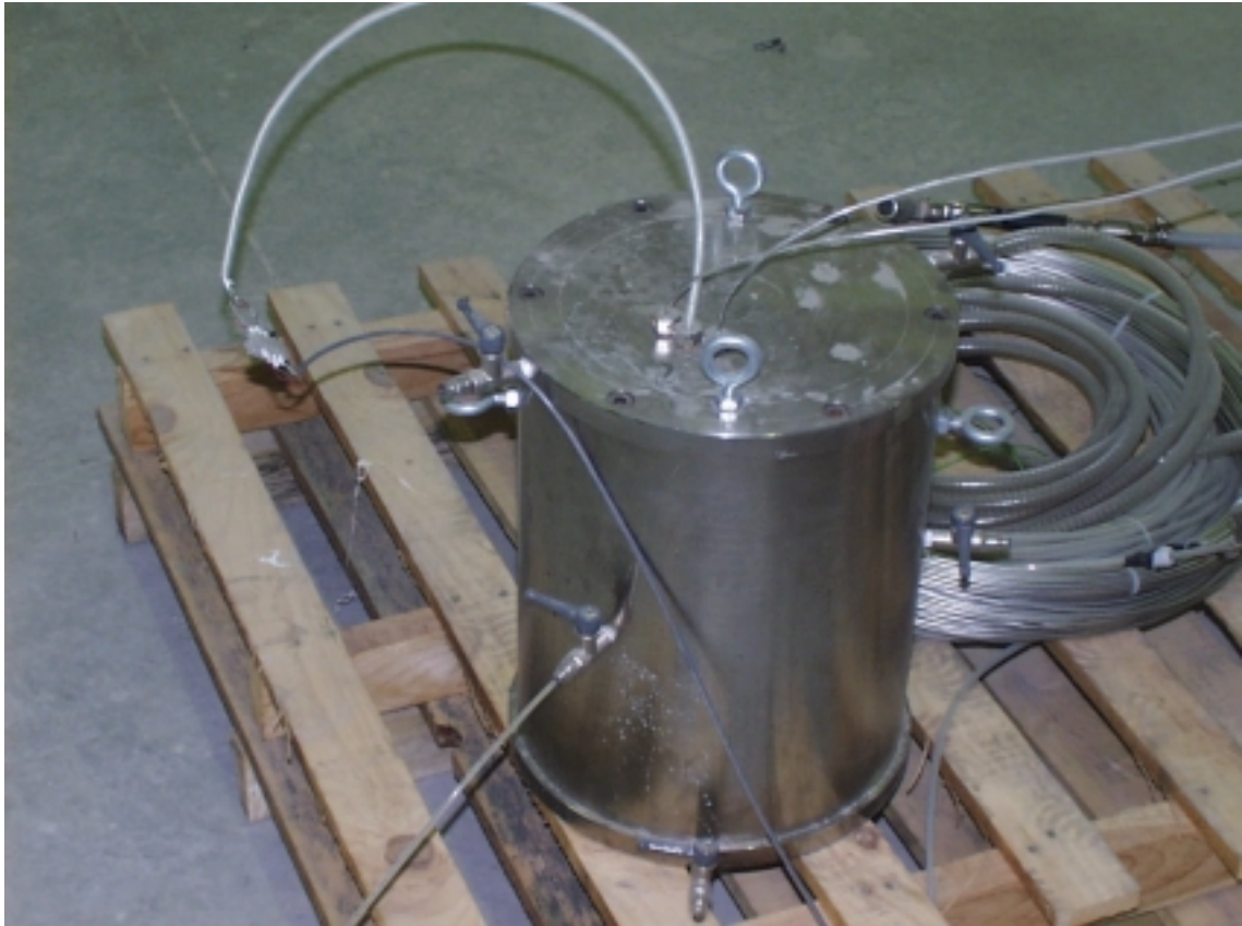
Figure 7-26. View of calibration cell.
