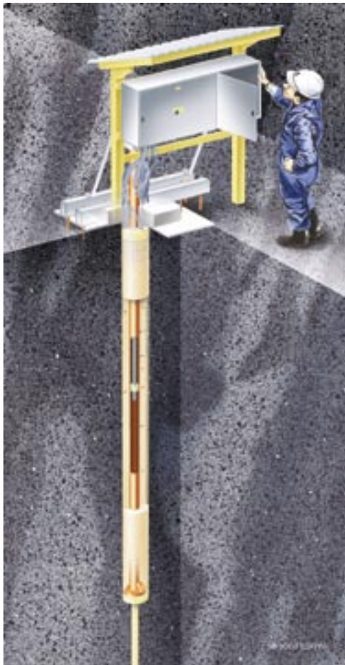
Figure 4-9. Illustration of the experimental set-up in the Long Term Test of Buffer Material (Lot) (left) and a cross-section view of one S-type parcel (right).
