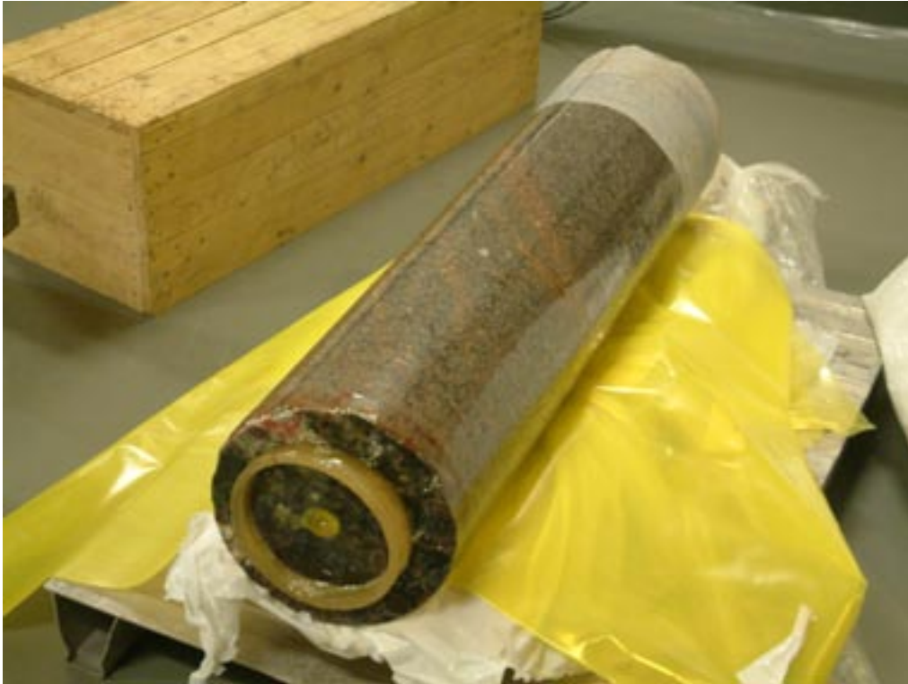
Figure 3-5. The 278 mm diameter core from LTDE-SD, including the 177 mm diameter core stub and rock surrounding the small diameter extension borehole. Core has been coated with epoxy resin to prevent cross-contamination during cutting and extraction of sample cores.
