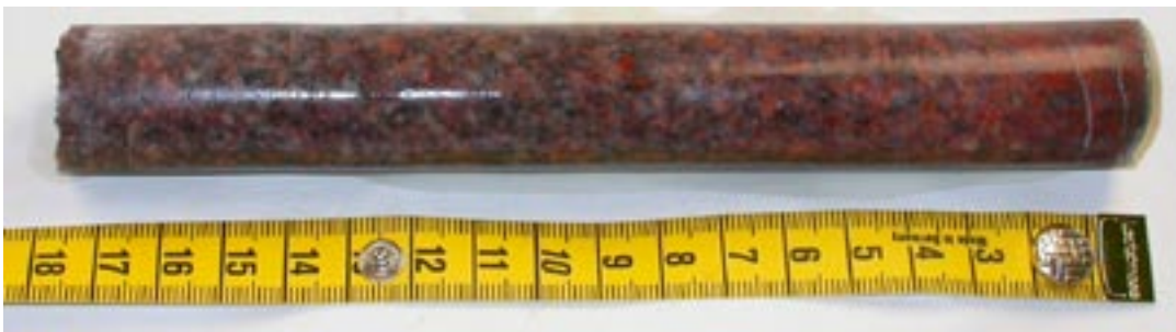
Figure 3-6. Sample core A6, about 18 cm long, drilled from the fracture surface on the core stub. Underneath the protective coating of epoxy resin a thin layer of calcite and chlorite is seen on the fracture surface. The rock is altered into about 4 cm from the fracture surface. Close to and in parallel to the fracture surface two fractures sealed with calcite are visible.
