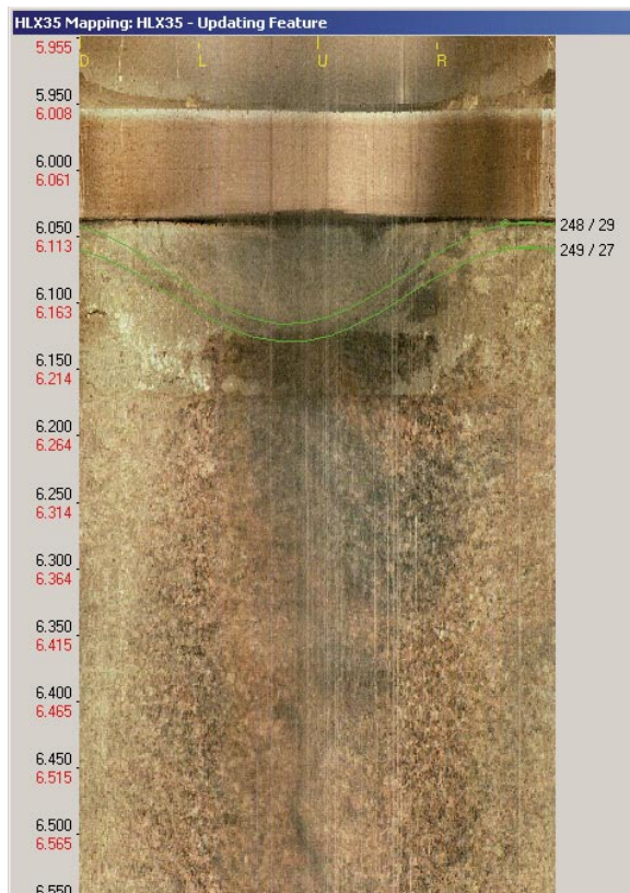
Figure 4-1. BIPS-image as seen in Boremap, borehole HLX35 showing the lowest part of the casing pipe, some rests of concrete from the bottom plug and the borehole wall. Rock type is Ävrö granite showing red staining (alteration) of medium intensity. Green lines mark the top of rock type and red staining. Vertical streaks are impurities on protective glass of BIPS-camera and light grey material is lowest part of the concrete seal /1/. Bottom of casing pipe is at 6.1 m.
