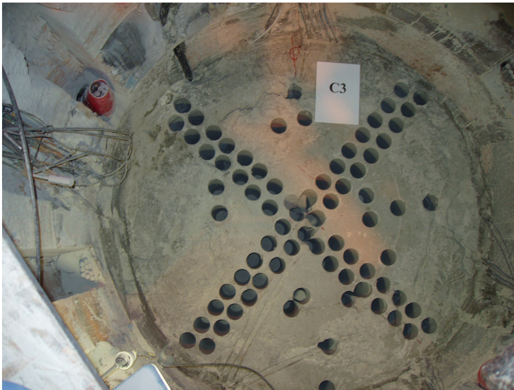
Figure 2-4. Cores taken from block C3.
