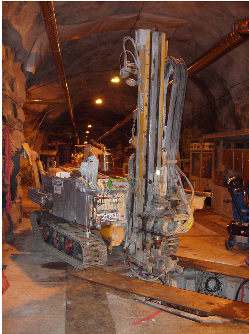
Figure 2-2. Type 705 DD drilling rig placed over the deposition hole.
