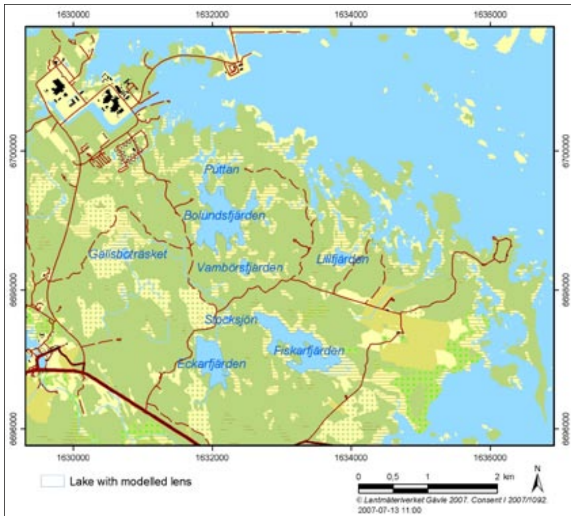
Figure 3-2. The eight lakes in the Forsmark area where lake sediment lenses have been modelled.
