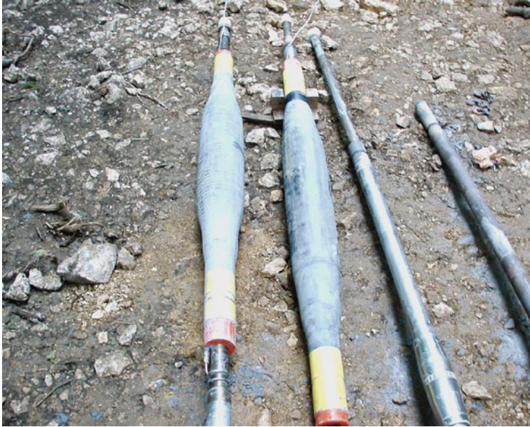
Figure 3-3. The straddled packer system showing its large deformability implying that it may operate in wells with very variable diameters.
