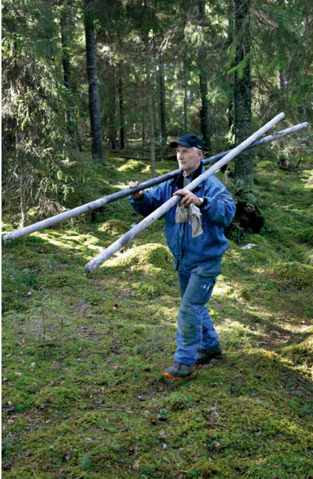
Another typical Forsmark phenomenon: Long, intact drill cores in three-metre lengths retrieved from the deep rock. Christian Steen carries drill cores from drilling site five at Bolundsfjärden.
