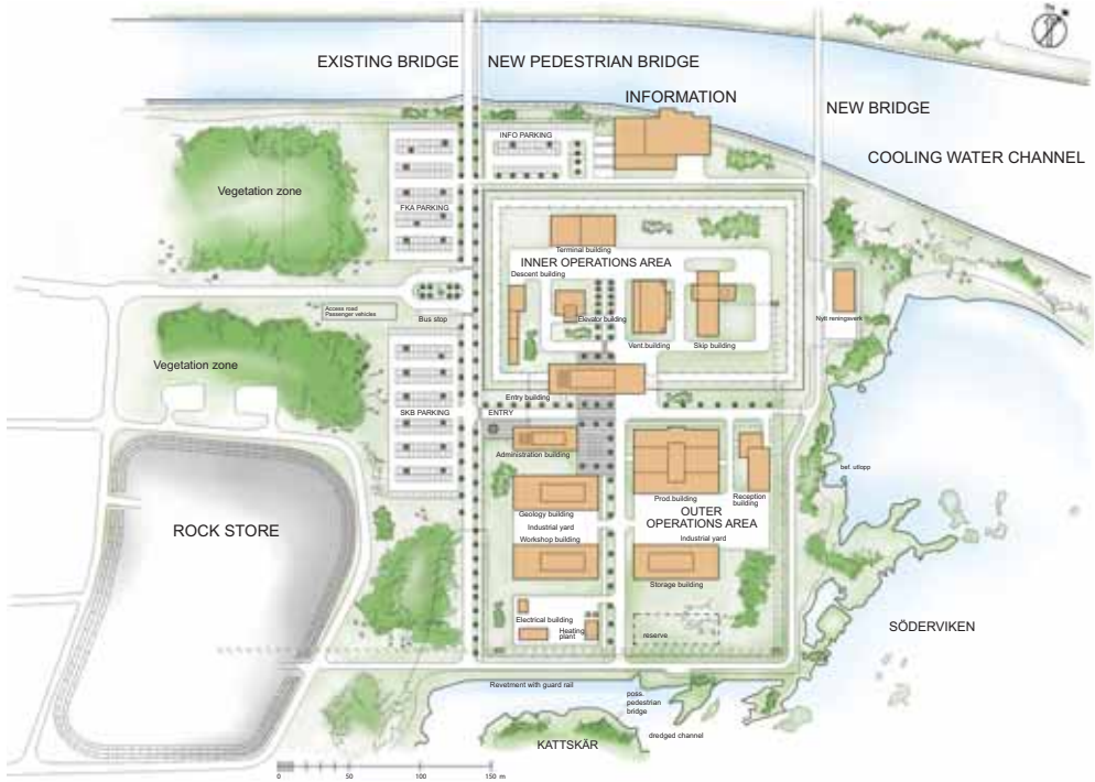
Preliminary site plan for an operations area on Söderviken, on the south side of the cooling water channel. A new bridge will be built between the existing bridge and the channel intake. A rock spoil heap may be located on land where parts of the barracks area are today.
