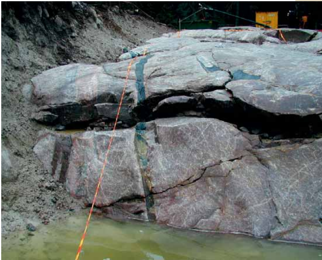
Example of a horizontal fracture filled with glacial sediments. The picture is from drilling site five. See drilling site map on page 108.
