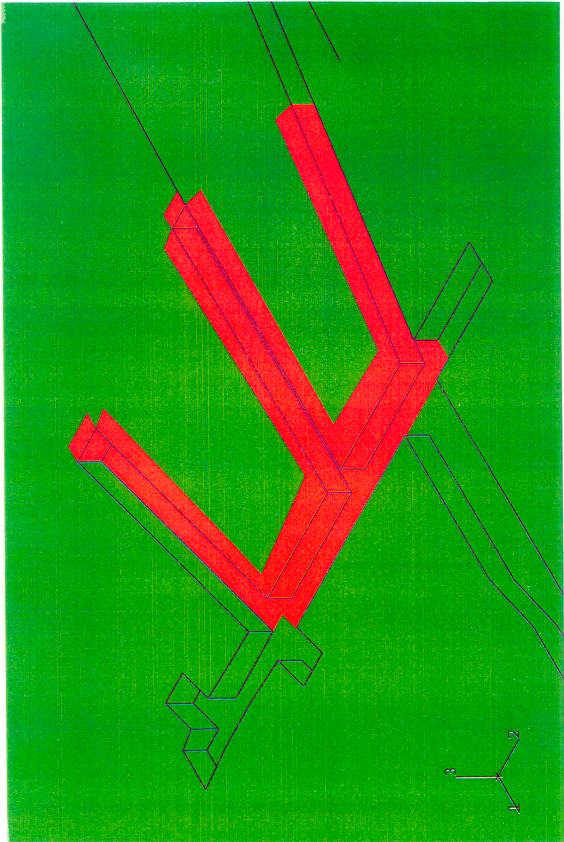
Figure 8-3. Skin zone with decreased hydraulic conductivity (red areas).
