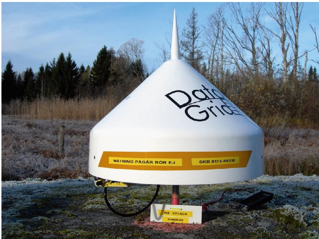
Figure 3-1. Sample station with choke ring antenna and GPS receiver mounted to the lower left. The station in this picture is PFM006489 but all sites have identical hardware (and firmware). They are mounted on a short steel rod anchored in the rock for good mechanical and thermal stability. However the low mounts increases the demand on the GPS environment. The antenna radome and pin are designed to protect the active components of the antenna and discourage birds and other small animals from lodging on the antenna. A second cover provides additional protection between measurement campaigns.
