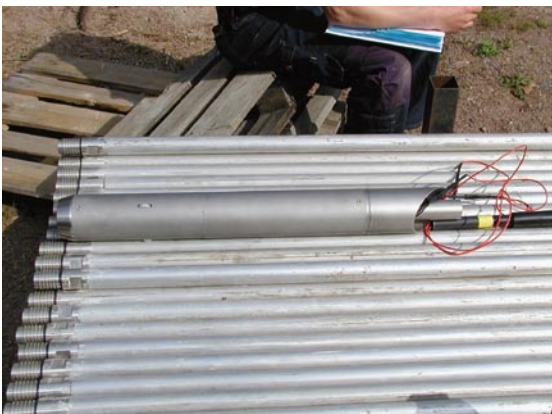
Photo 5. Positioner, bottom end of down-in-hole string.
