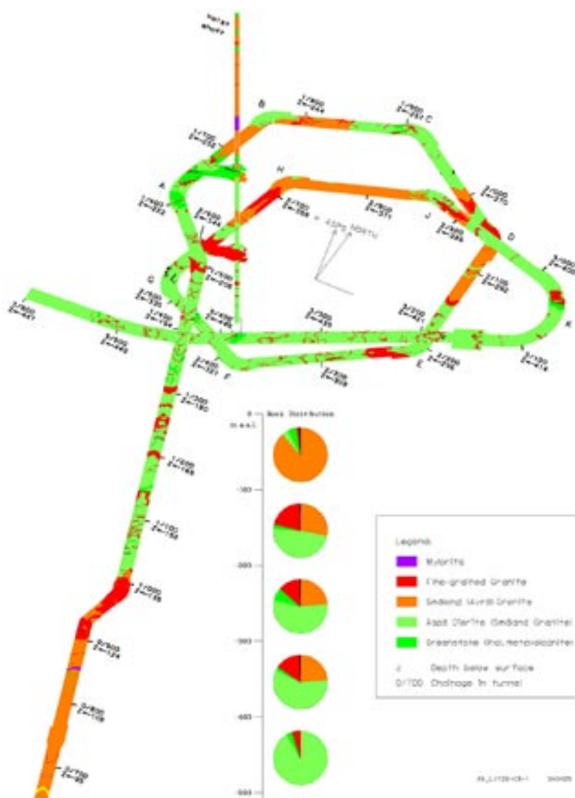
Figure 3-6. Simplified bedrock map of Äspö including the underground structures /Andersson and Söderhäll 2001/.
