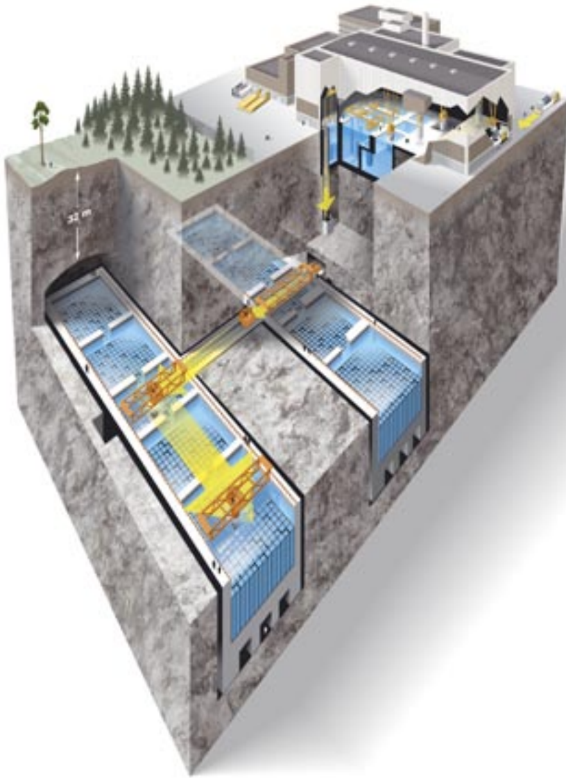
Figure 5-1. Layout of the Clab 1 and 2 showing the surface facilities and underground structures.
