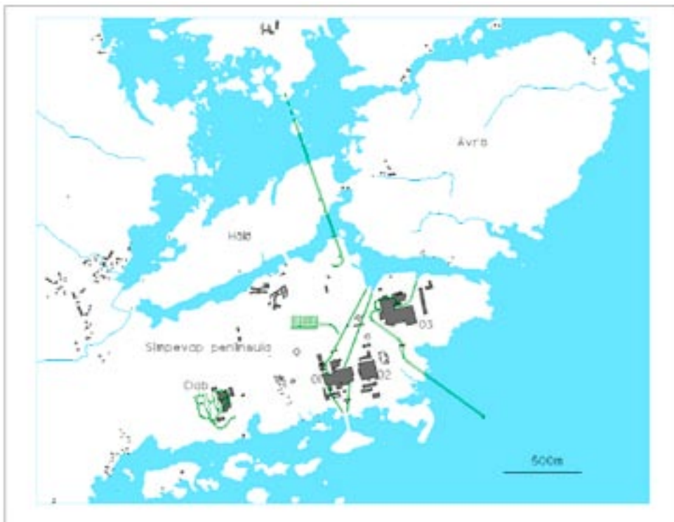
Figure 1-1. A plan view of the project area showing the major projects. The underground structures are shown in green colour /Curtis et al. 2003/.
