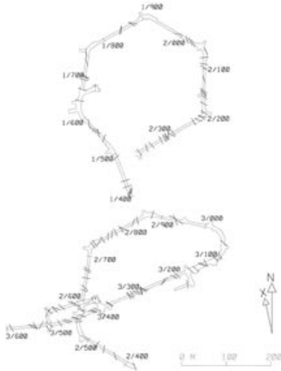
Figure 6-12. Mapped large, single, open, water bearing fractures in the tunnel. The fractures are mainly sub-vertical. N = Magnetic North, x = North in the Äspö coordinate system /Rhén et al. 1997b/.
