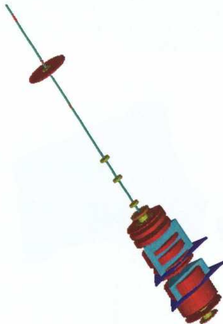
Figure 3-7. A set of borehole parameters visualised by lines (rock type), cylinders (rock quality) and triangular tubes (water leakage).
