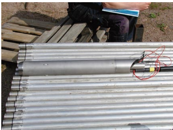
Photo 5. Positioner, bottom end of down-hole string.
