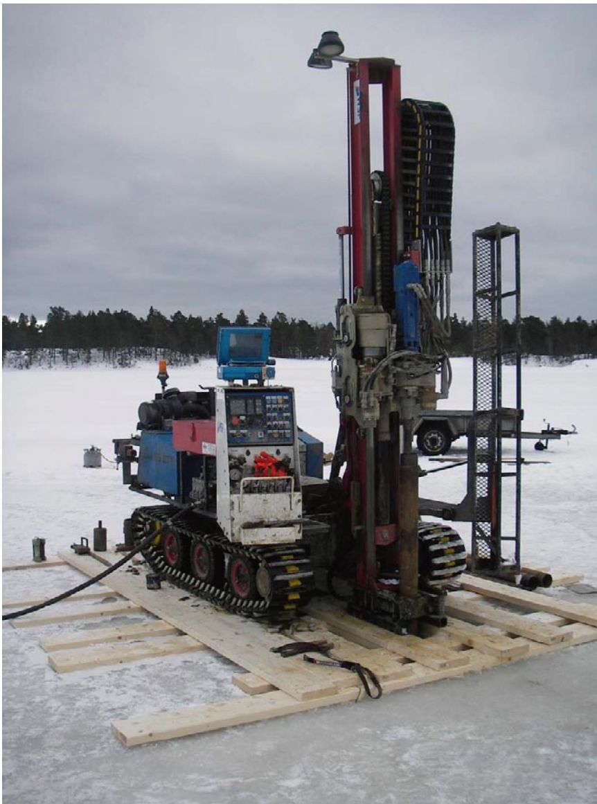
Figure 3-1. GM 65 GTT drilling rig on seawater ice.
