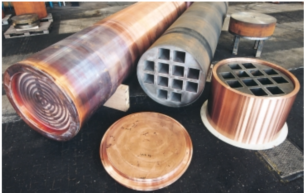
Figure 7-7. Finished parts from trial fabrication of canisters.
