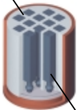
Figure 3-2. Canister for spent nuclear fuel.
