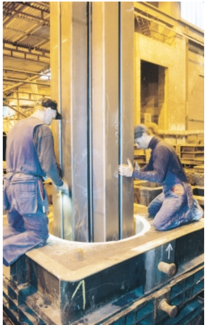
Figure 7-8. A welded cassette for BWR fuel is placed in the mould.
