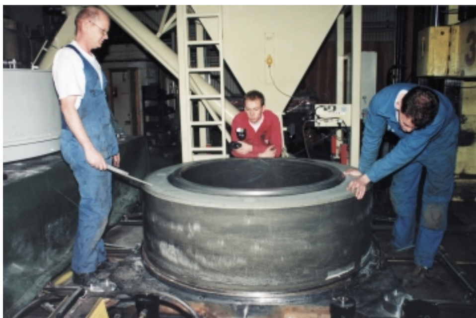
Figure 7-5. Ring-shaped bentonite block on a full scale (outside diameter 1.65 m, height 0.5 m) fabricated by uniaxial pressing. Blocks of this type will be used for the full-scale trials at the Äspö HRL.
