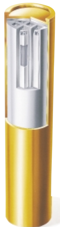
Figure 7-1. Copper canister with insert of cast iron for BWR fuel.
