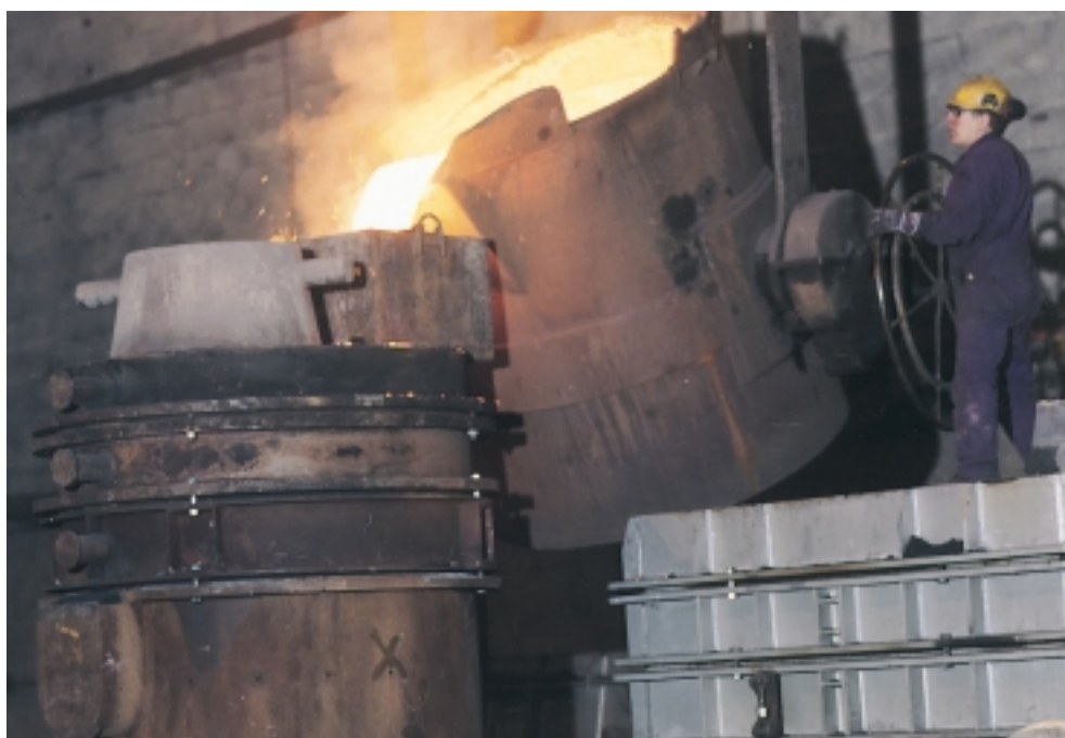
Figure 7-9. The mould is filled with molten iron.
