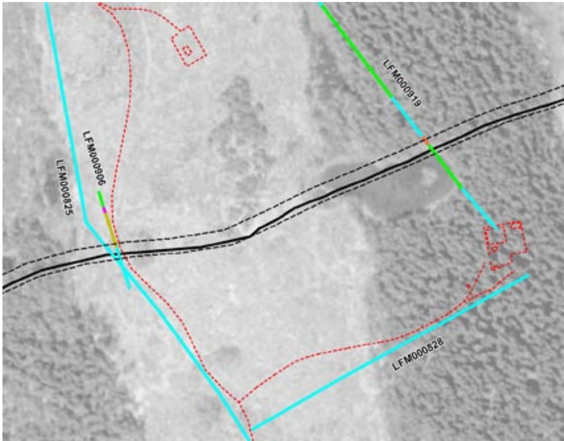
Figure 5-2. Refraction seismic profiles LFM000825 (5 m geophone spacing) and LFM000906 (2 m geophone spacing) traversing the inferred deformation zone ZFMENE0060A (black dashed lines) and low magnetic lineament MF0060A0 (black solid line) close to drill sites 1 and 5. Magnitude of bedrock velocity as in Figure 5-1. Roads and drill sites are shown with a red dashed line. The profile LFM000906 is 100 m long. Background, GSD-ortofoto © Lantmäteriet, Gävle 2001, Permission M2001/5268.
