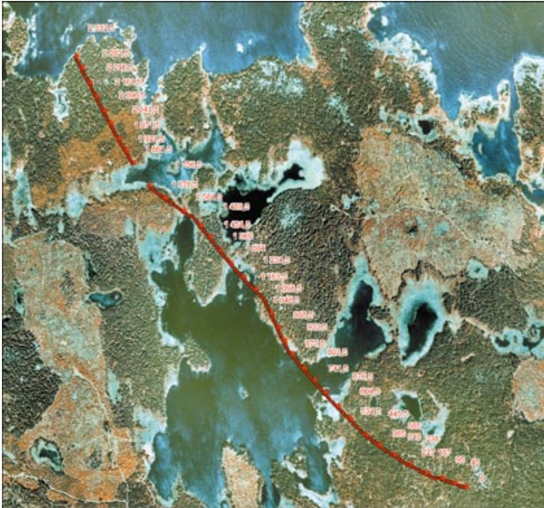
Figure 1-1. Location of the refraction seismic profile LFM001017. Labels denote section length coordinates in metres along the profile.
