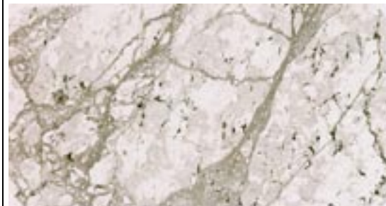
Scanned thin-section of fracture network in core segment at 268.2 m. Chlorite and epidote group minerals fill the space between the angular fragments (after SKB P-06-212)
