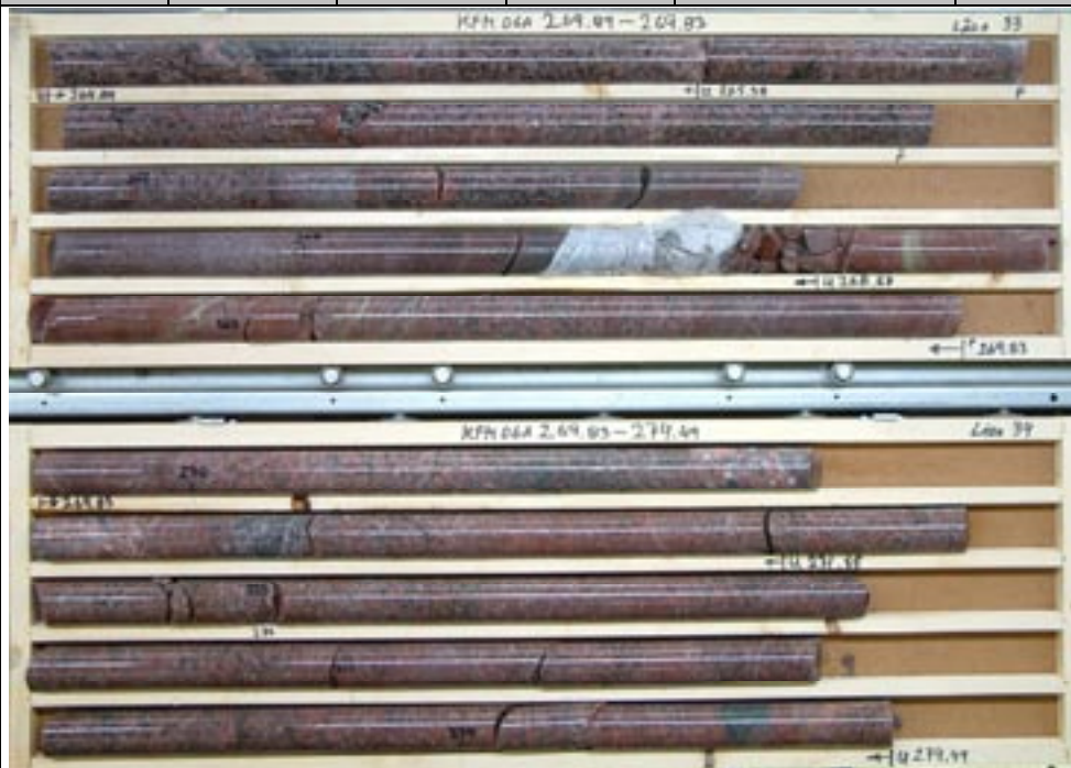
KFM06A (DZ3). Strong alteration (red-stained bedrock with hematite dissemination) and abundant sealed fractures are present
