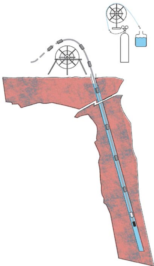
Figure 3-1. Equipment for Hydrochemical logging in boreholes. At the lower end of the tube array there is a non-return valve and a weight connected. Each tube unit is 50 m long.
