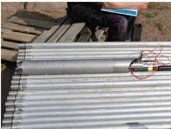
Photo 5. Positioner, bottom end of down-in-hole string.
