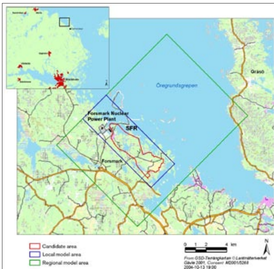
Figur 3-1. The Forsmark area with environs. The extents of the regional (green) and local (blue) model areas as well as of the candidate area (red) are outlined in the map.
