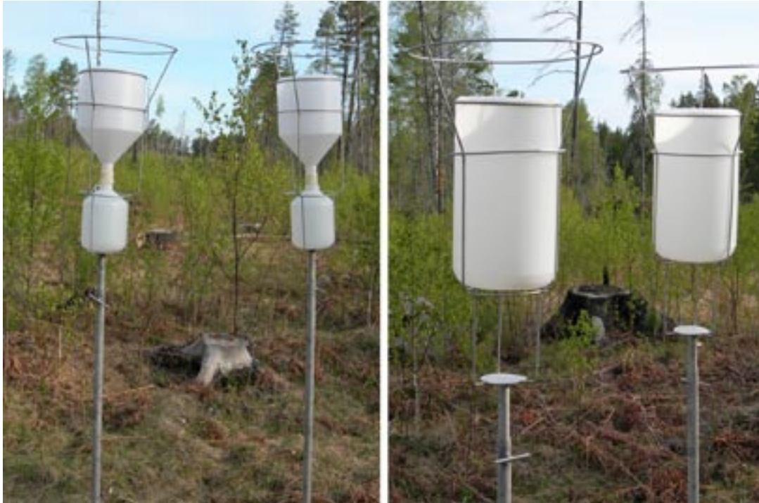
Figure 4-24. Sample collectors for precipitation (PFM002564), to the left for rain and to the right for snow. The construction prevents evaporation.
