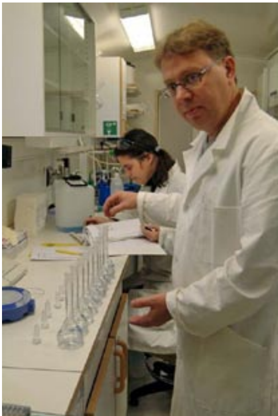
Figure 4-25. Indoor picture from the SKB mobile field laboratory. The laboratory is mainly used for time critical analyses (pH, EC, alkalinity, Fe(tot), Fe(+II) and ammonium) and for certain treatment/preservation of water samples.
