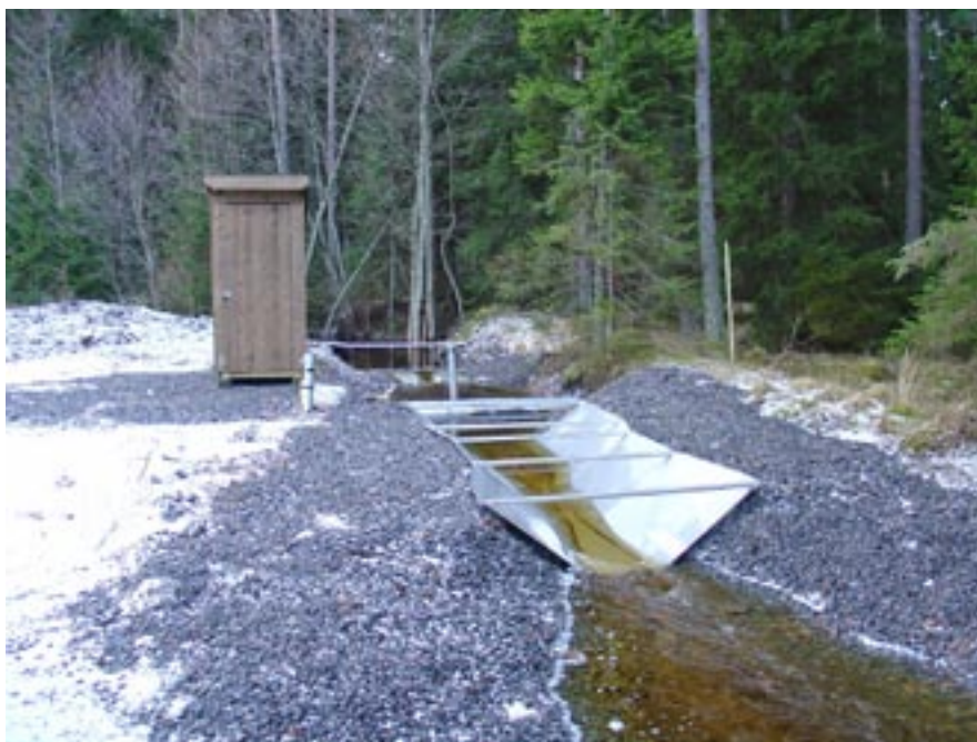
Figure 4-7. Discharge station PFM002667 with the large flume in the foreground, the small flume upstream in the background, and the service module to the left. The tube in the middle of the brook between the flumes is screened and used for installation of devices for measurement of electrical conductivity and temperature.
