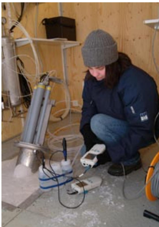
Figure 4-23. During the field measurements of pH, temperature and conductivity, water from the borehole is led through a measurement cell consisting of three plastic bottles.
