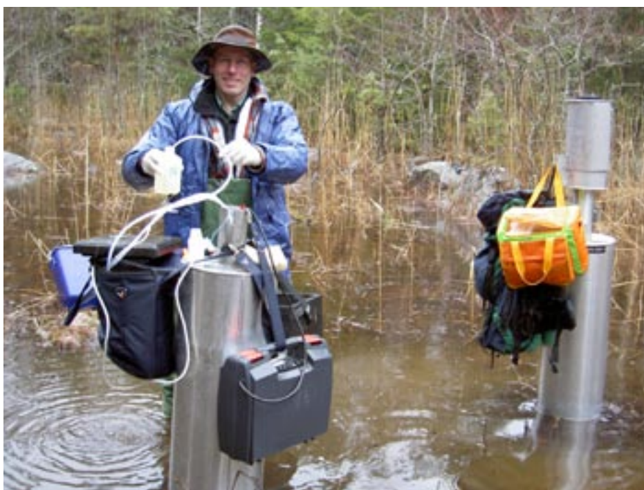
Figure 4-21. Sampling of shallow groundwater in soil pipes driven into sediments below the surface water table in a wetland at Forsmark.
