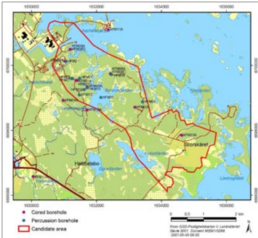
Figure 4-22. Locations of percussion- (blue) and core drilled boreholes (red) included in the hydro-chemical monitoring programme.
