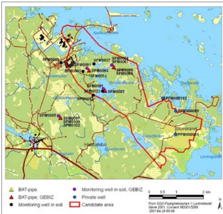
Figure 4-20. Locations of soil pipes, pipes supplied with BAT-type filter tips, and private wells. Objects belonging to the GEBIZ-programme (see explanation in Table 4-10) are shown as red and purple in filled triangles and circles, respectively.
