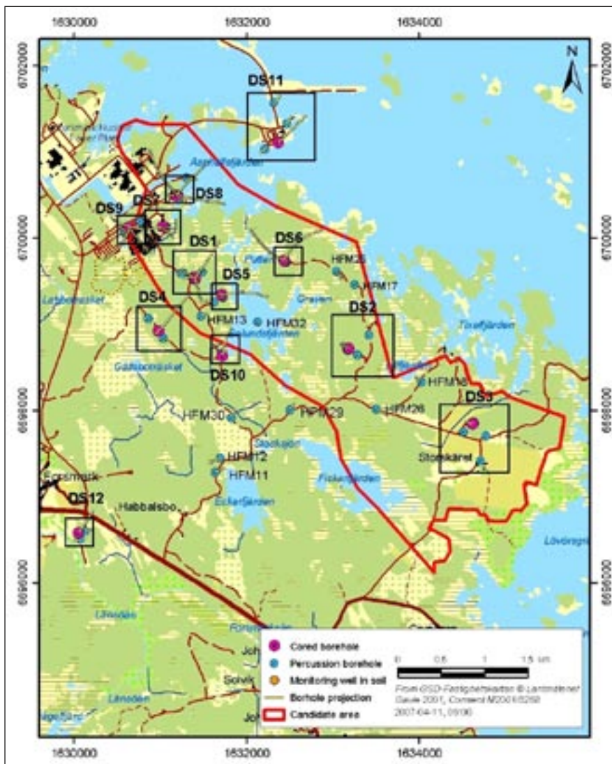
Figure 3-2. The localization within and close to the Forsmark candidate area of all twelve drill sites for core drilled boreholes. The map also exhibits most of the percussion drilled boreholes completed during the site investigations, in connection to as well as outside these drill sites. Details of the drill sites are given in Figure 3-3.
