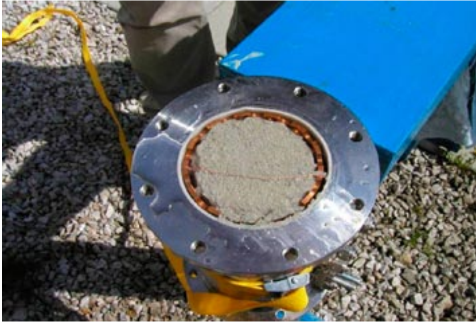
Figure 4-26. Laboratory and small-scale field testing of erodability of clay components in perforated tubes.
