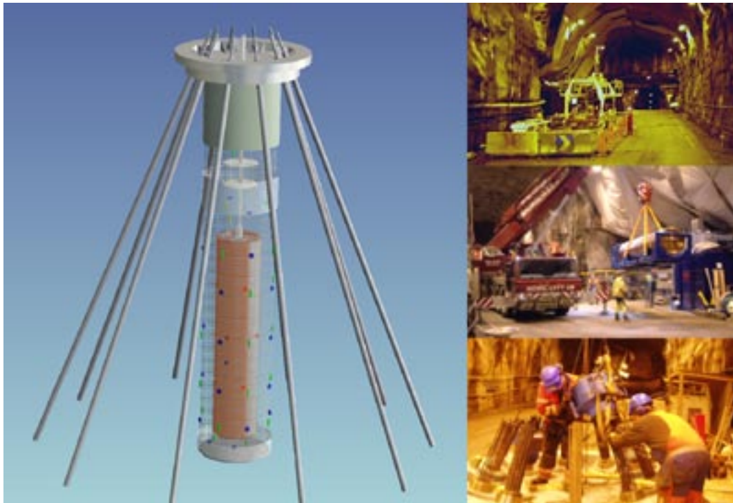
Figure 4-24. Layout of the Lasgit experiment showing the copper canister, the bentonite buffer, the location of some of the instrumentation, the plug and rock anchors. From top to bottom the photographs on the right-hand side show the assembly hall area, the movement of the copper canister prior to installation and the pre-tensioning of the steel lid.
