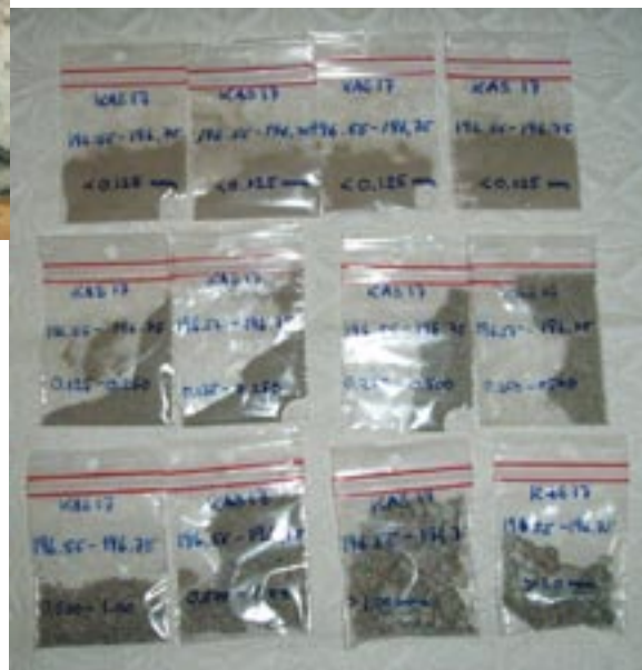
Figure 3-17. Photo of sample from a fracture zone at 196.55–196.75 m in borehole KAS17.
