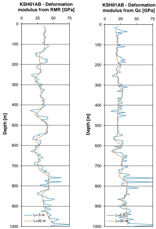
**Figure 2-11.** KSH01AB: Variation of the deformation modulus from RMR (left) and  $Q_c$  (right) depending on the core section length adopted for the rock mass characterisation. Results for core sections of 5 and 30 m are shown.
