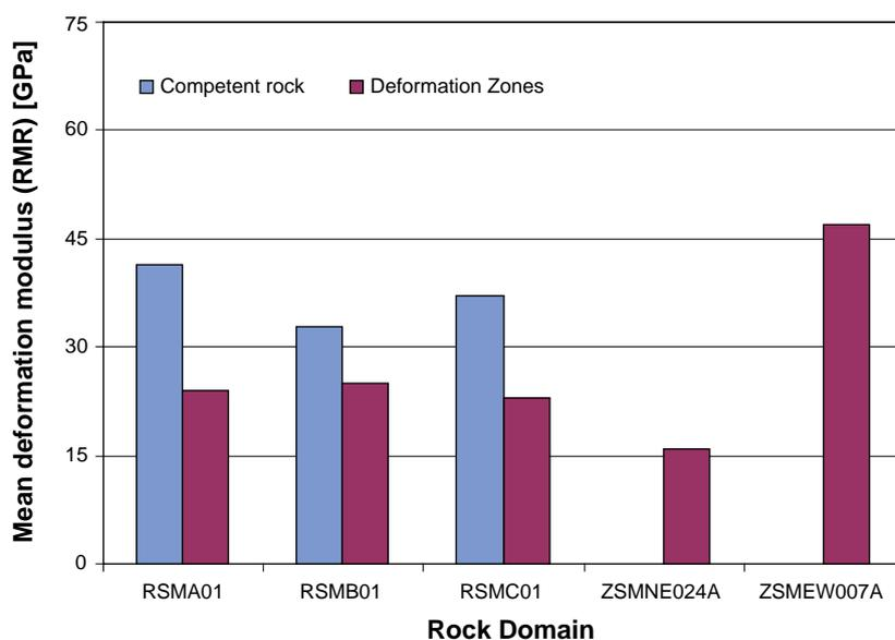
**Figure 4-2.** Mean deformation modulus from RMR of the rock mass in Rock Domain RSMA01, RSMB01 and RSMC01 (“competent” and “deformation” zones) and for Deterministic Deformation Zone ZSMNE024A and ZSMEW007A in Simpevarp SDM v. 1.2.
