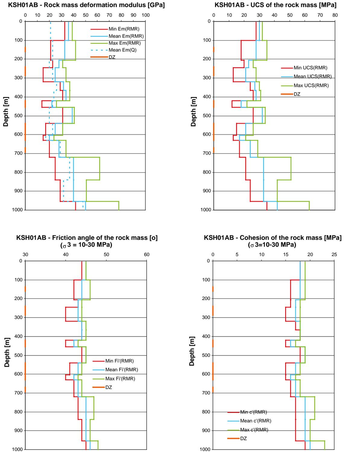
**Figure 2-6.** KSH01AB: Variation of the deformation modulus, uniaxial compressive strength, friction angle and cohesion of the rock mass with depth. The minimum, mean and maximum values are shown for each rock unit in the geological “single-hole interpretation”.
