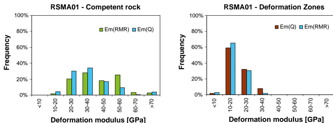
**Figure 4-1.** Histogram of the deformation modulus of the rock mass determined from Q and RMR for the competent rock (left) and fractured rock/deformation zones (right) in Rock Domain RSMA01 in Simpevarp SDM v. 1.2.
