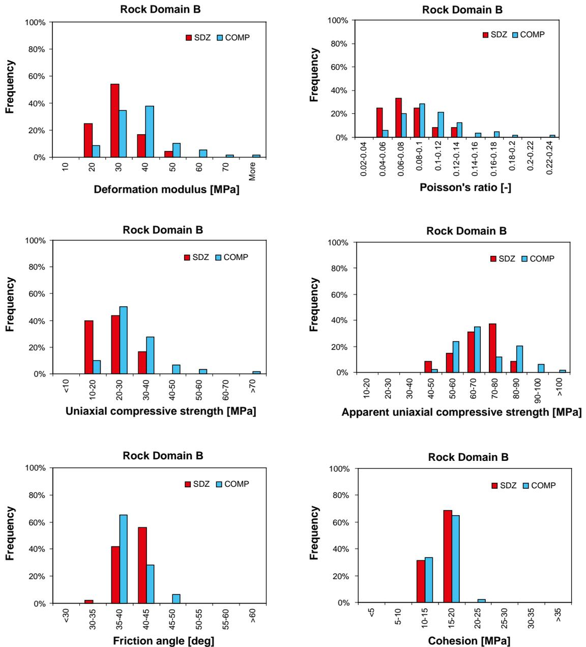
**Figure A1-9.** Rock Domain RSMB01: Histograms of the deformation modulus Poisson's ratio, uniaxial compressive strength, apparent uniaxial compressive strength, friction angle and cohesion of the rock mass determined by means of RMR for the competent rock (COMP) and fractured rock (SDZ). In this figure, the histograms for ZSMEW007A are not reported because they are only based on one value for each property.
