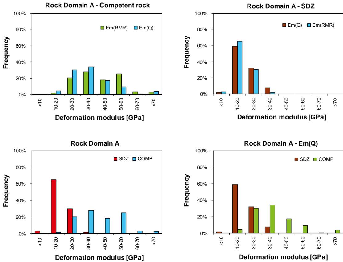
*Figure A1-5. Rock Domain RSMA01: Histograms showing the comparison of the results from RMR and Q for the competent rock (COMP) and fractured rock (SDZ), respectively. In this figure, the histograms for ZSMEW007A are not reported because they are only based on one value for each property.*
