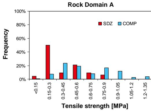
**Figure AI-7.** Rock Domain RMSA01: Histogram of the tensile strength of the rock mass determined by means of RMR for the competent rock (COMP) and fractured rock (SDZ). In this figure, the histograms for ZSMEW007A are not reported because they are only based on one value for each property.
