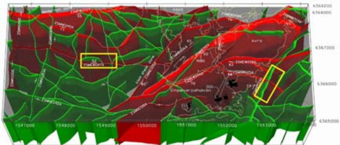
**Figure 3-2.** Simpevarp v. 1.2 Local Model Volume with the indication of the high confidence (in red) and possible (in green) Deterministic Deformation Zones. Zone ZSMNE024A and ZSMEW007A are highlighted in yellow.
