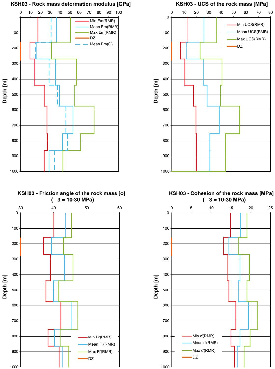
**Figure 2-8.** KSH03A: Variation of the deformation modulus, uniaxial compressive strength, friction angle and cohesion of the rock mass with depth. The minimum, mean and maximum values are shown for each rock unit in the geological “single-hole interpretation”.
