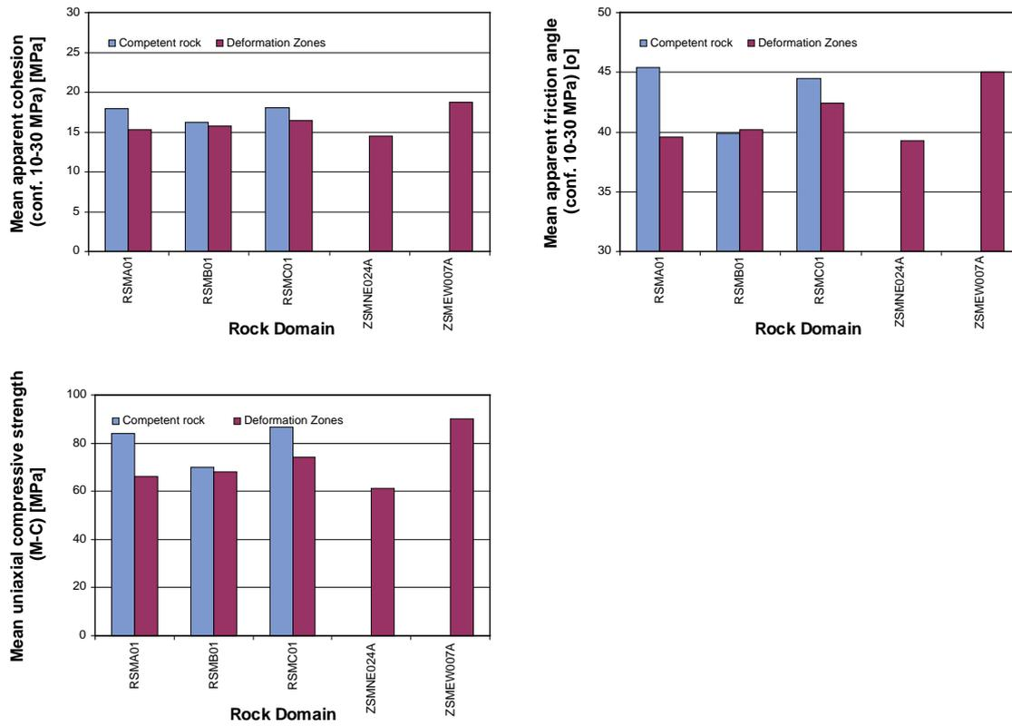
*Figure A1-2. Rock Mechanics properties of the Rock Domains and Deformation Zones for Simpevarp Site Descriptive Model v. 1.2. The mean apparent cohesion, friction angle and uniaxial compressive strength of the rock mass according to Mohr-Coulomb's Criterion are illustrated.*
