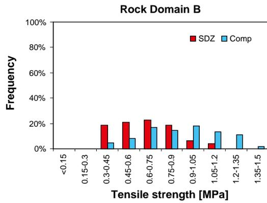
**Figure A1-10.** Rock Domain RSMB01: Histogram of the tensile strength of the rock mass determined by means of RMR for the competent rock (COMP) and fractured rock (SDZ). In this figure, the histograms for ZSMEW007A are not reported because they are only based on one value for each property.
