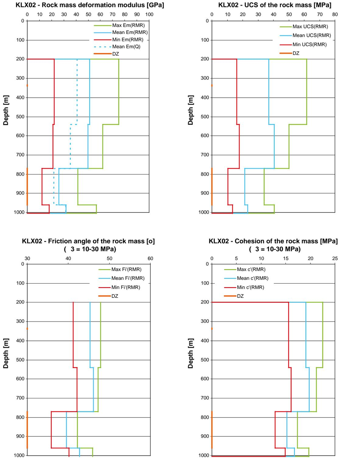
**Figure 2-10.** KLX02: Variation of the deformation modulus, uniaxial compressive strength, friction angle and cohesion of the rock mass with depth. The minimum, mean and maximum values are shown for each rock unit in the geological “single-hole interpretation”.
