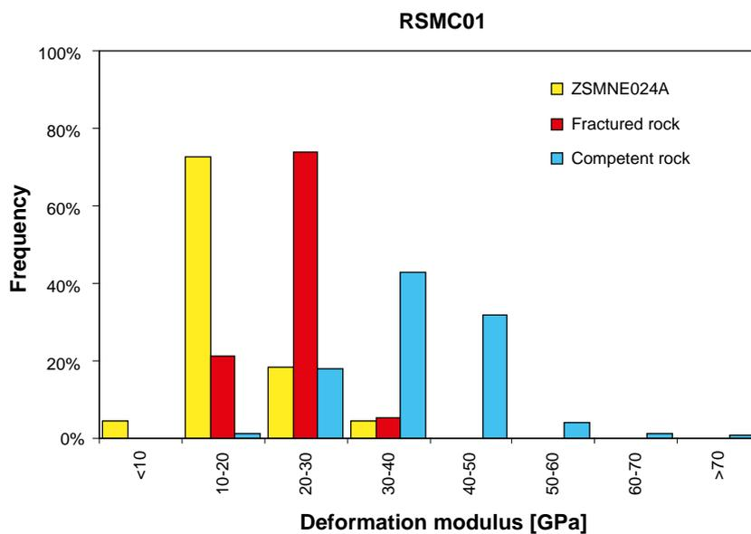
**Figure 4-4.** Histogram of the deformation modulus of the rock mass in Rock Domain RSMC01 (competent and fractured rock/deformation zones) and Deterministic Deformation Zone ZSMNE024A.
