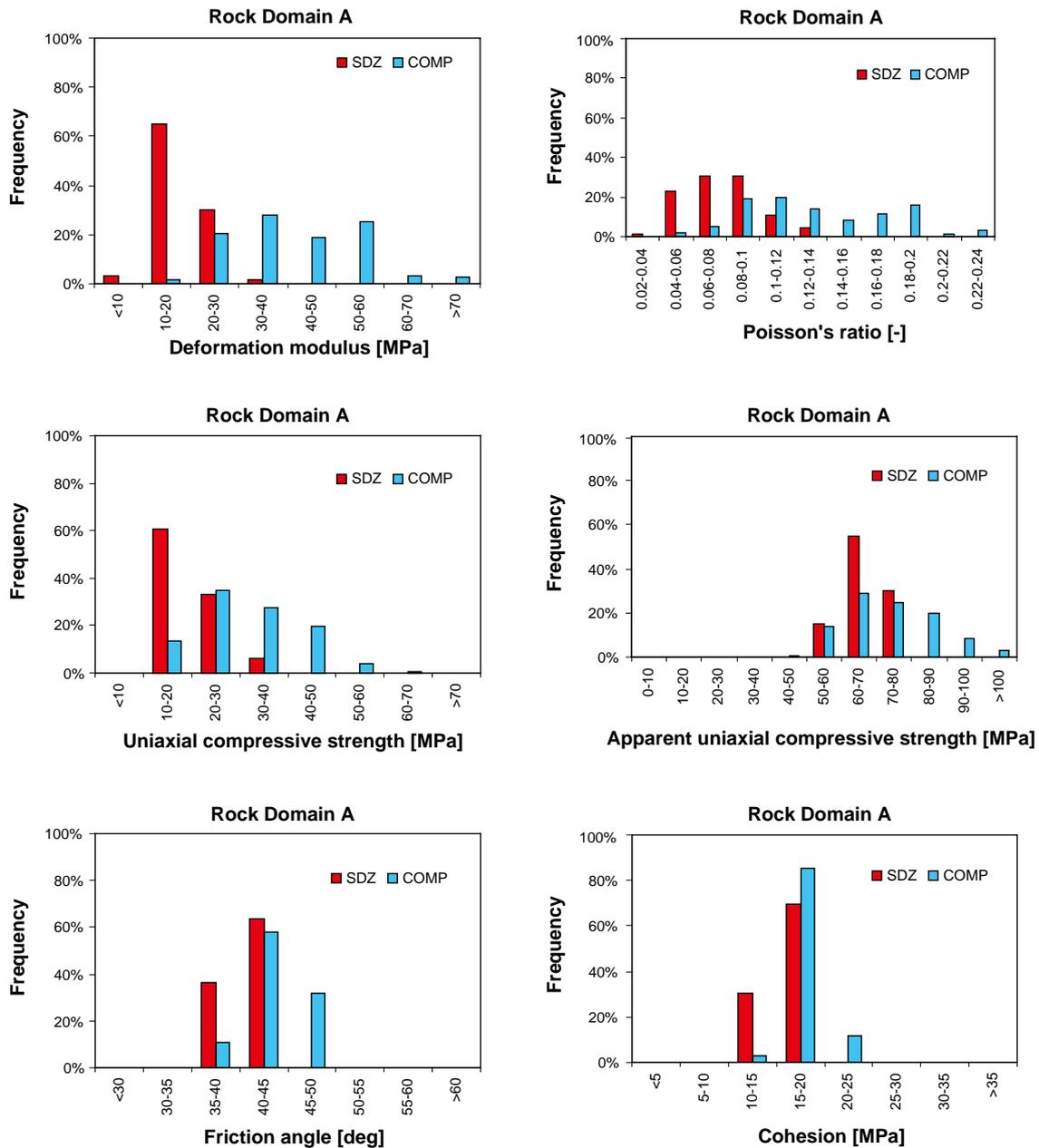
**Figure A1-6.** Rock Domain RMSA01: Histograms of the deformation modulus, uniaxial compressive strength, apparent uniaxial compressive strength, friction angle and cohesion of the rock mass determined by means of RMR for the competent rock (COMP) and fractured rock (SDZ). In this figure, the histograms for ZSMEW007A are not reported because they are only based on one value for each property.
