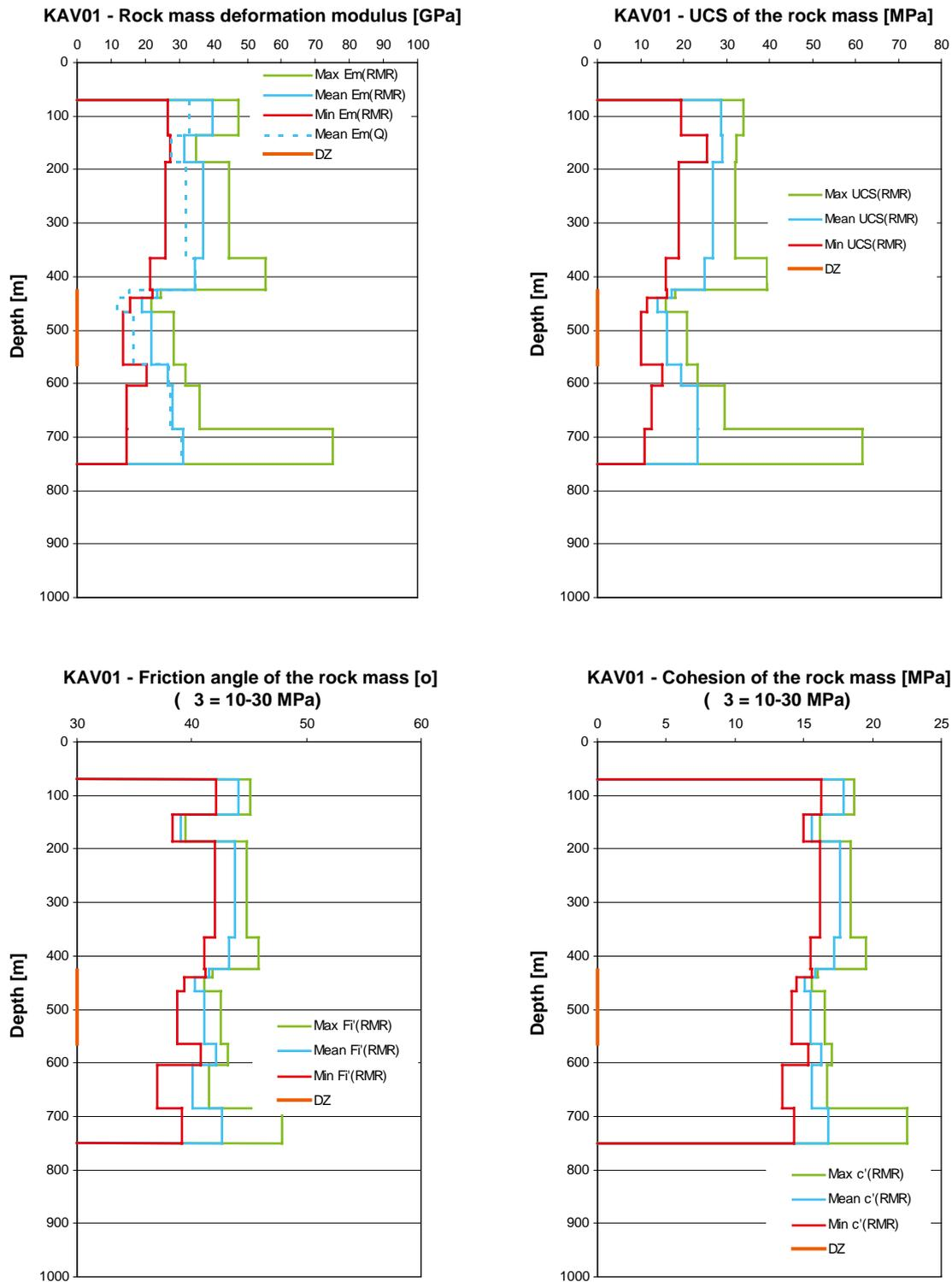
**Figure 2-9.** KAV01: Variation of the deformation modulus, uniaxial compressive strength, friction angle and cohesion of the rock mass with depth. The minimum, mean and maximum values are shown for each rock unit in the geological “single-hole interpretation”.
