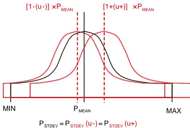
**Figure 3-3.** Description of the statistical distribution and uncertainty of the Rock Mechanics parameters determined by means of the Empirical Approach.
