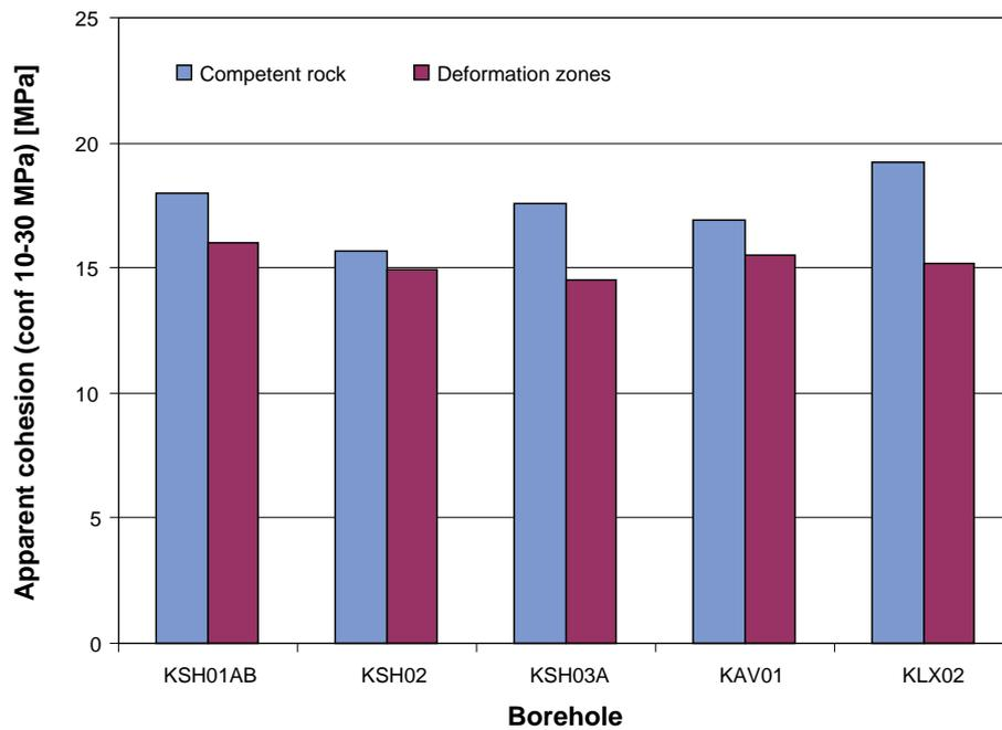
*Figure 2-5. Mean apparent cohesion of the rock mass for the analysed boreholes. The average values for competent rock and deformation zones are shown. The confinement stress is between 10 and 30 MPa. Please note that the fractured rock in KSH03AB corresponds to the Deterministic Deformation Zone ZMSNE024A.*
