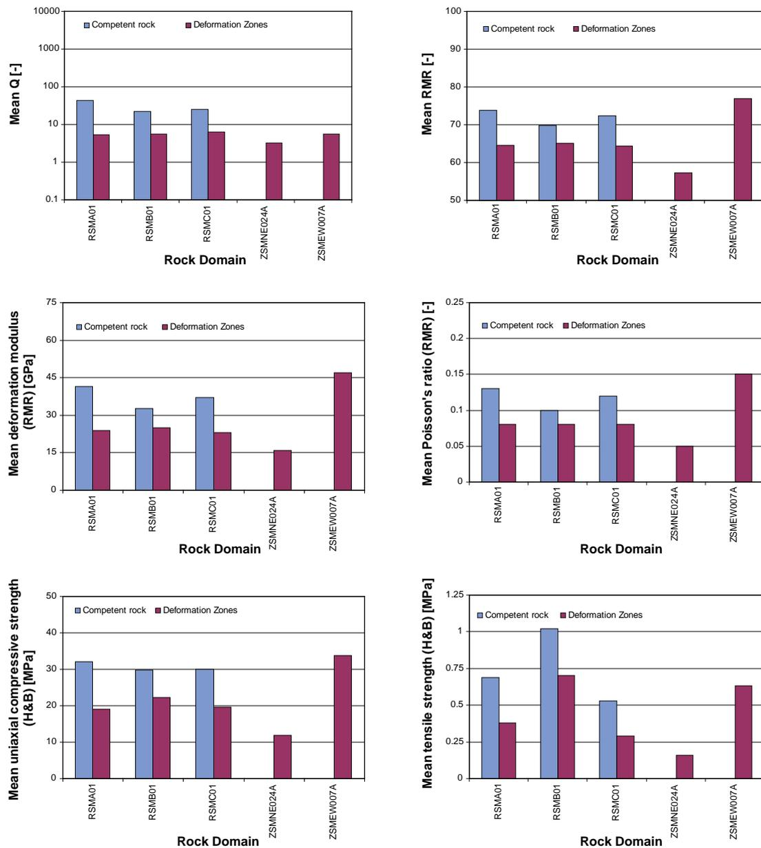
Figure A1-1. Rock Mechanics properties of the Rock Domains and Deformation Zones for Simpevarp Site Descriptive Model v. 1.2. The mean  $Q$  and RMR values, the deformation modulus and Poisson's ratio, the uniaxial and tensile strength according to Hoek & Brown's Criterion are illustrated for the competent and fractured rock mass.
