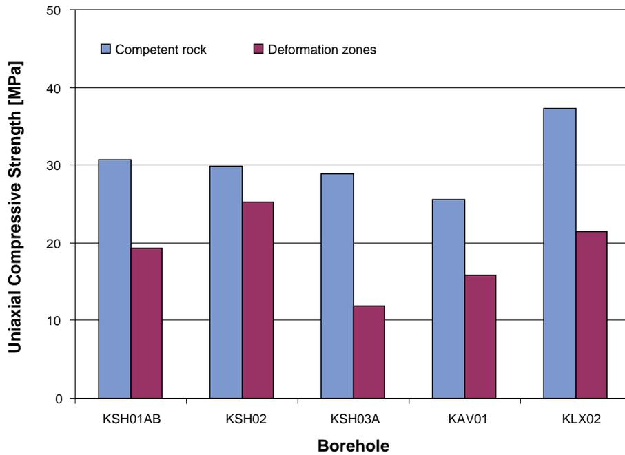
*Figure 2-3. Mean uniaxial compressive strength of the rock mass according to Hoek & Brown's Criterion for the analysed boreholes. The average values for competent rock and deformation zones are shown. Please note that the fractured rock in KSH03AB corresponds to the Deterministic Deformation Zone ZMSNE024A.*
