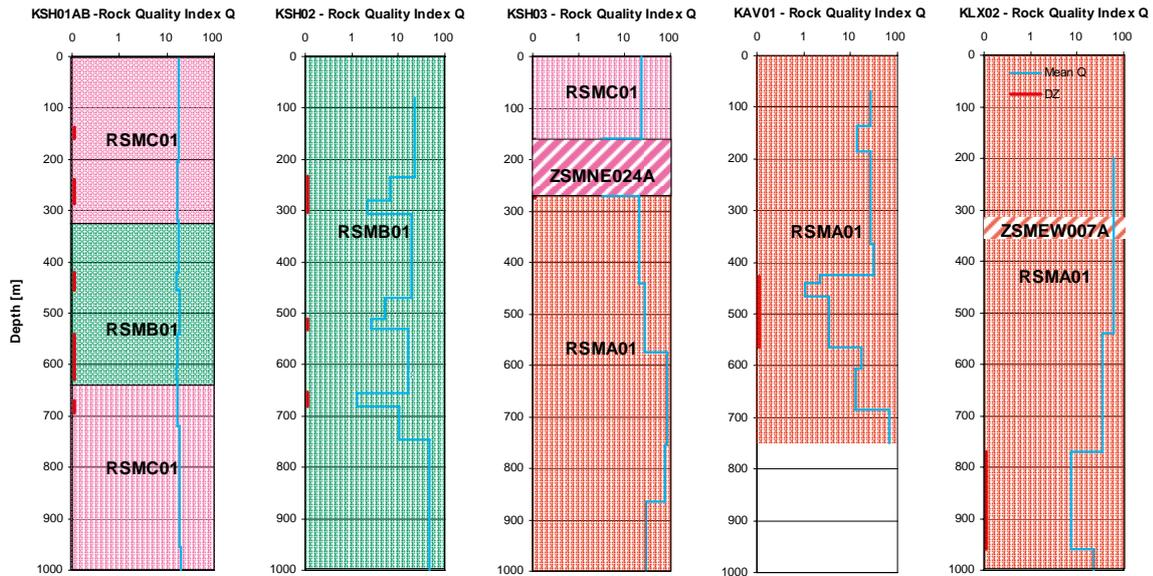
**Figure 3-1.** Partitioning of the boreholes into Rock Domains and Deformation Zones. The mean  $Q$  value is also plotted along the boreholes.
