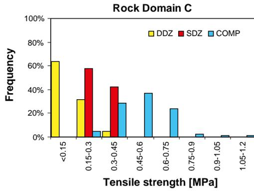
**Figure A1-13.** Rock Domain RSMC01: Histogram of the tensile strength of the rock mass determined by means of RMR for the competent rock (COMP), fractured rock (SDZ) and the deterministic Deformation Zone (DDZ) ZMSNE024A. In this figure, the histograms for ZSMEW007A are not reported because they are only based on one value for each property.
