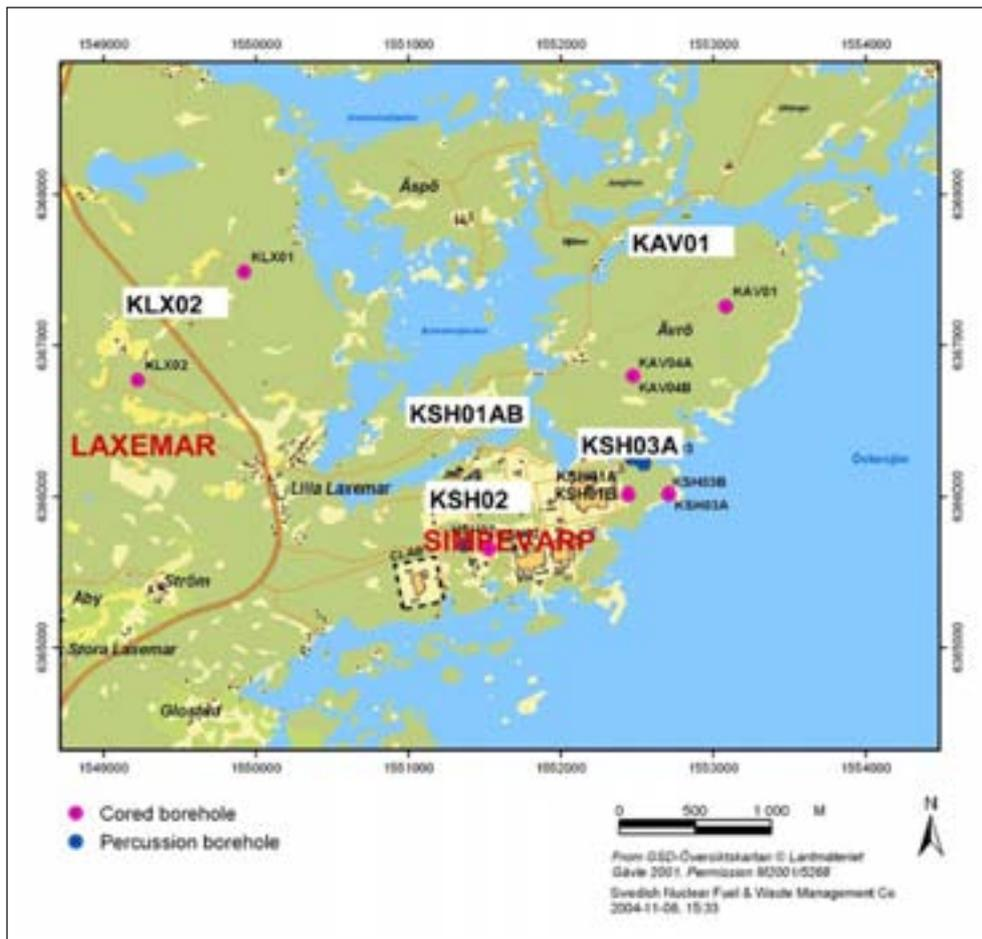
Figure 1-1. Overview of the Simpevarp and Laxemar Sites with indication of borehole KSH01AB, KSH02, KSH03A, KAV01 and KLX02 used for the Rock Mechanics characterisation.
