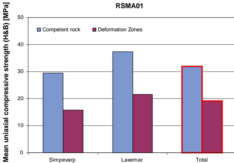
**Figure 4-3.** Equivalent uniaxial compressive strength of the rock mass in Rock Domain RSMA01 for Simpevarp, Laxemar, and for the whole Model Volume.
