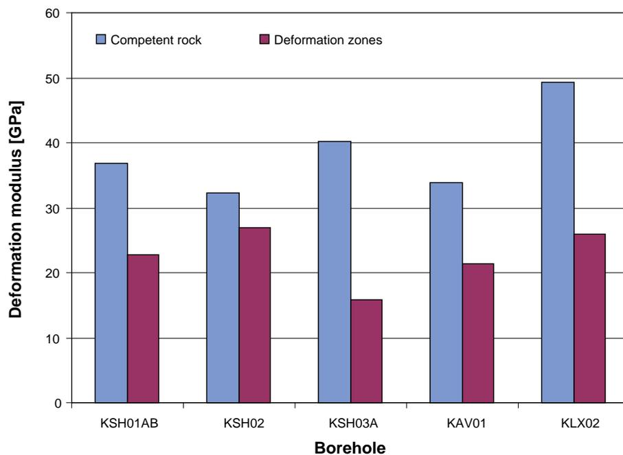
**Figure 2-2.** Mean deformation modulus of the rock mass for the analysed boreholes. The average values for competent rock and deformation zones are shown. Please note that the fractured rock in KSH03AB corresponds to the Deterministic Deformation Zone ZMSNE024A.
