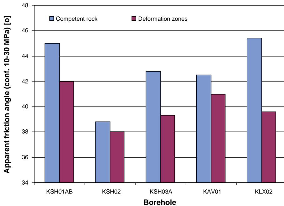
*Figure 2-4. Mean apparent friction angle of the rock mass for the analysed boreholes. The average values for competent rock and deformation zones are shown. The confinement stress is between 10 and 30 MPa. Please note that the fractured rock in KSH03AB corresponds to the Deterministic Deformation Zone ZMSNE024A.*
