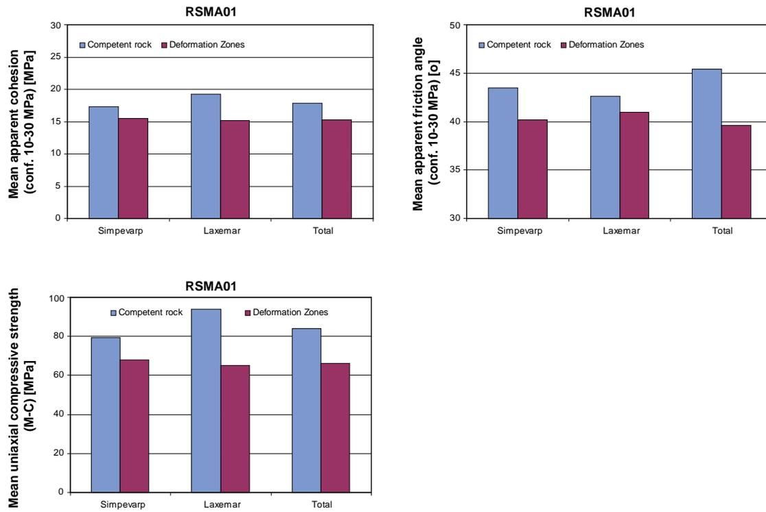
*Figure A1-4. Rock Mechanics properties of the competent rock and deformation zones for Rock Domain RSMA01 of Simpevarp Site Descriptive Model v. 1.2. The mean apparent cohesion, friction angle and uniaxial compressive strength of the rock mass according to Mohr-Coulomb's Criterion are illustrated.*
