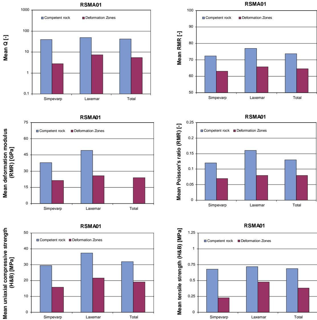
*Figure A1-3. Rock Mechanics properties of the competent rock and deformation zones for Rock Domain RSMA01 of Simpevarp Site Descriptive Model v. 1.2. The mean  $Q$  and RMR values, the deformation modulus and Poisson's ratio, the uniaxial and tensile strength according to Hoek & Brown's Criterion are illustrated for the competent and fractured rock mass.*
