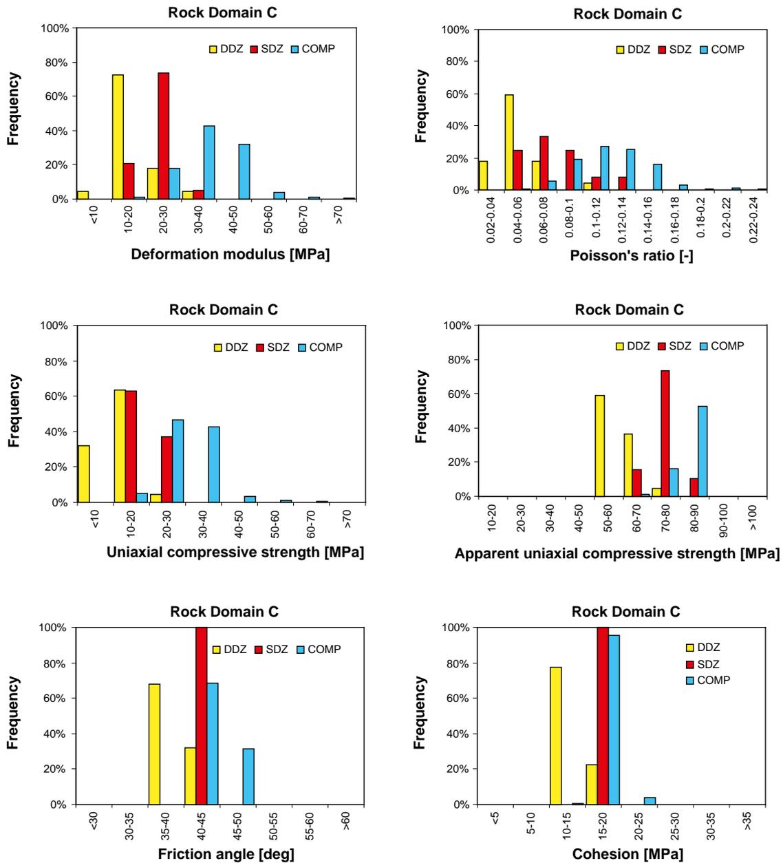
**Figure A1-12.** Rock Domain RSMC01: Histograms of the deformation modulus Poisson's ratio, uniaxial compressive strength, apparent uniaxial compressive strength, friction angle and cohesion of the rock mass determined by means of RMR for the competent rock (COMP), fractured rock (SDZ) and the deterministic Deformation Zone (DDZ) ZMSNE024A. In this figure, the histograms for ZSMEW007A are not reported because they are only based on one value for each property.
