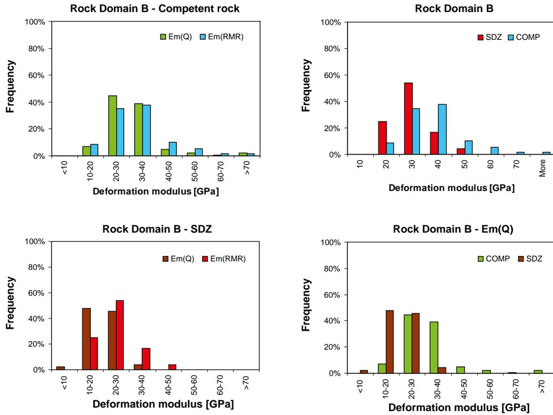
*Figure A1-8. Rock Domain RSMB01: Histograms showing the comparison of the results deformation modulus from RMR and Q for the competent rock (COMP) and fractured rock (SDZ), respectively. In this figure, the histograms for ZSMEW007A are not reported because they are only based on one value for each property.*
