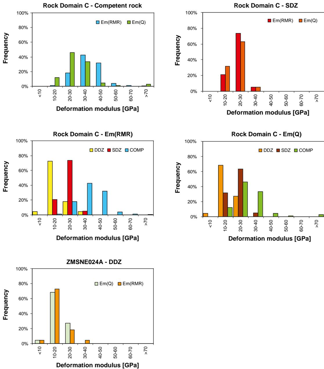
**Figure A1-11.** Rock Domain RSMC01: Histograms showing the comparison of the results of deformation modulus from RMR and Q for the competent rock (COMP), fractured rock (SDZ) and the deterministic Deformation Zone (DDZ) ZMSNE024A, respectively. In this figure, the histograms for ZSMEW007A are not reported because they are only based on one value for each property.
