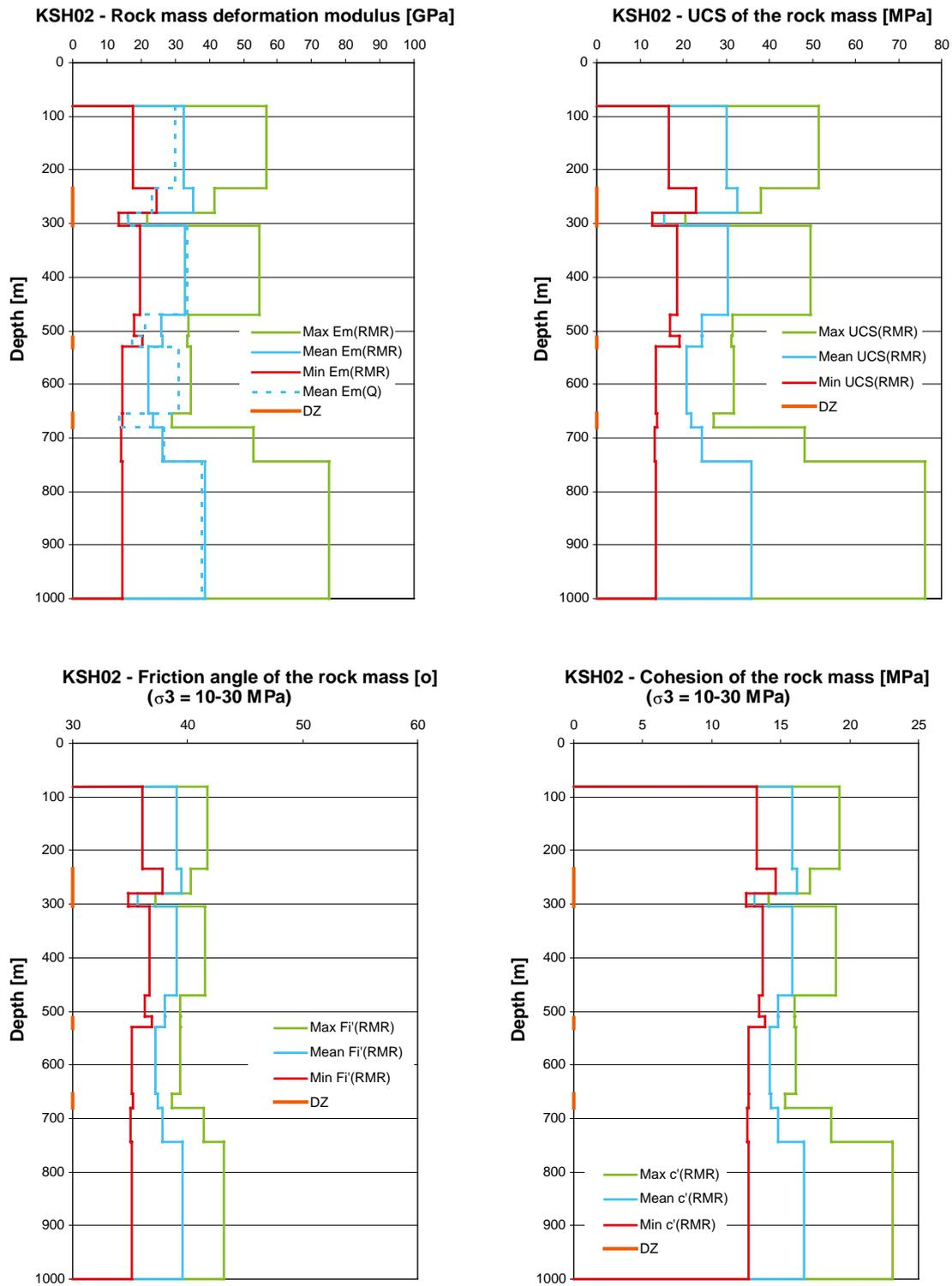
*Figure 2-7. KSH02: Variation of the deformation modulus, uniaxial compressive strength, friction angle and cohesion of the rock mass with depth. The minimum, mean and maximum values are shown for each rock unit in the geological “single-hole interpretation”.*
