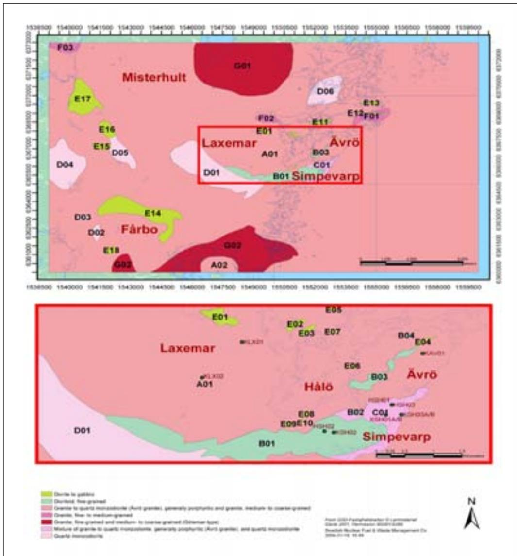
**Figure 2-1.** Map of the Rock Domains in the Simpevarp v. 1.2 Regional and Local Model Volume. 36 Rock Domains appear in the Regional Model, of which 17 are included in the Local Model.
