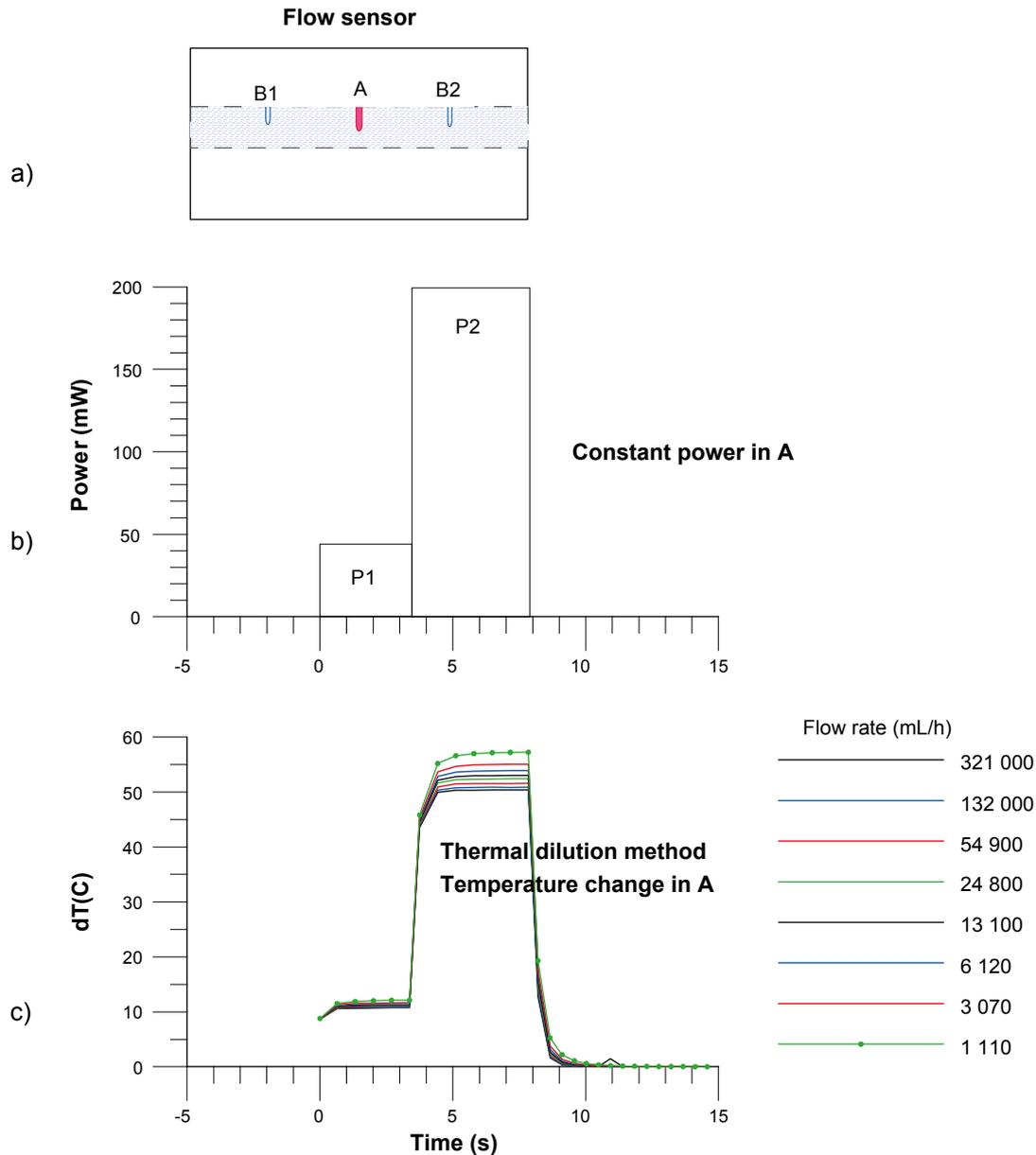
**Figure 3-4.** Flow measurement, flow rate > 600 mL/h.
