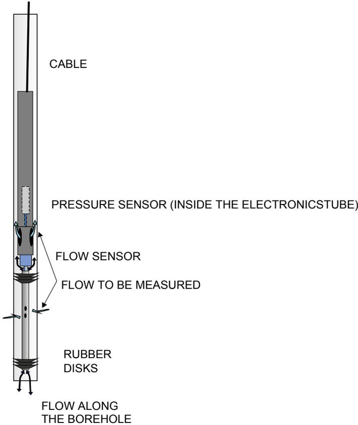
**Figure 3-2.** The absolute pressure sensor is located inside the electronics tube and connected through a tube to the borehole water.
