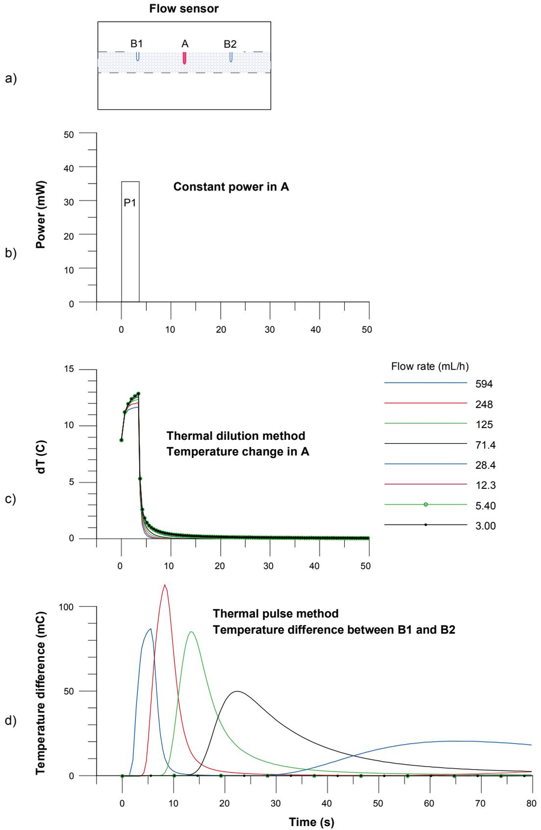
*Figure 3-3. Flow measurement, flow rate < 600 mL/h.*
