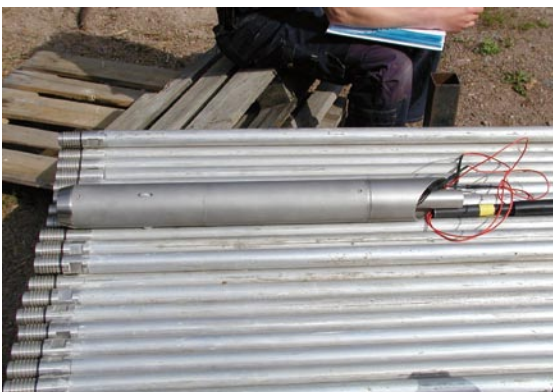
Photo 5. Positioner, bottom end of down-in-hole string.
