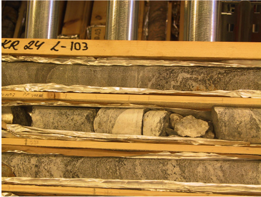
Plate IV. Borehole depths 396-400 m (Levels -386 to -390). Fracture-rich zone. Photo: R. Pusch.
