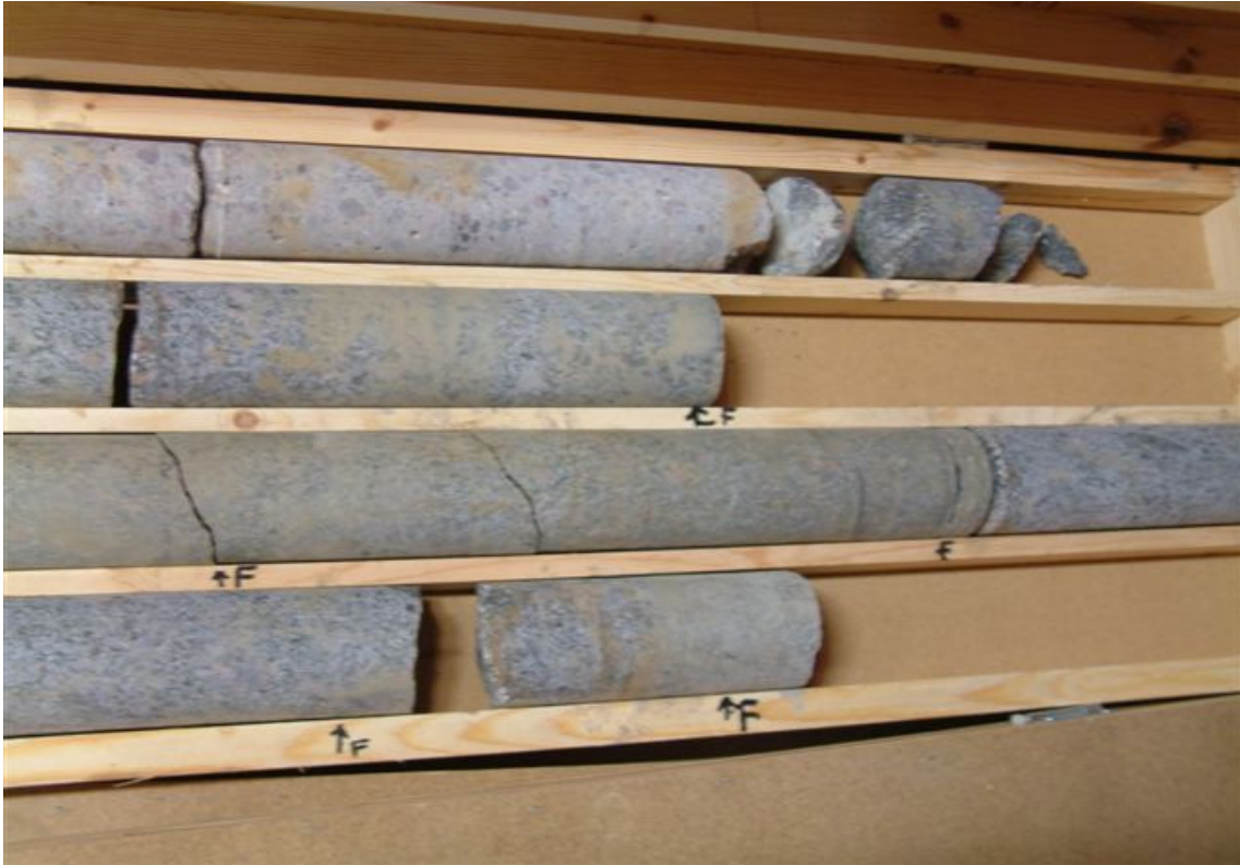
Figure 3-3. Hole KA1621G01. The core representing the lower 2-3 meters of the hole has at least 3 water-bearing fractures.
