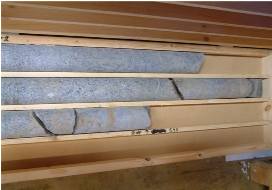
Figure 3-4. Hole KA1621G02. The core representing the lower 3 meters of the hole has at least 3 water-bearing fractures.
