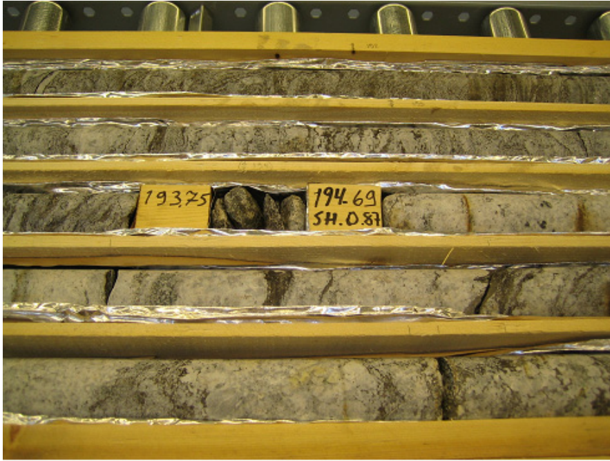
Plate II. Borehole depths 194-196 m (Levels -184 to -186). Fracture-rich part just below depth 194.7 m (Level -184.7). Photo: R. Pusch.
