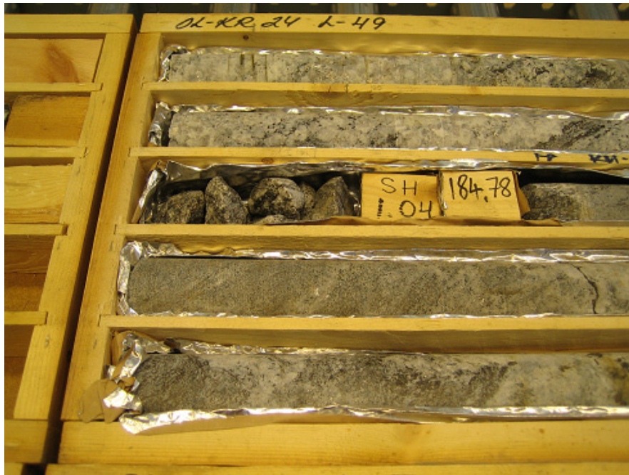
Plate I. Depth 184-186 m/ (Level -174 to -176). Fracture-rich part just below depth 185 m (Level -175). Photo: R.Pusch.
