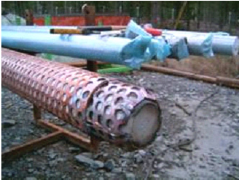
Figure 2-5. Lower ends of clay plug units. End of segment to be placed on solid concrete plug. In the background: Plug units wrapped in tight plastic for protecting them from moisture.
