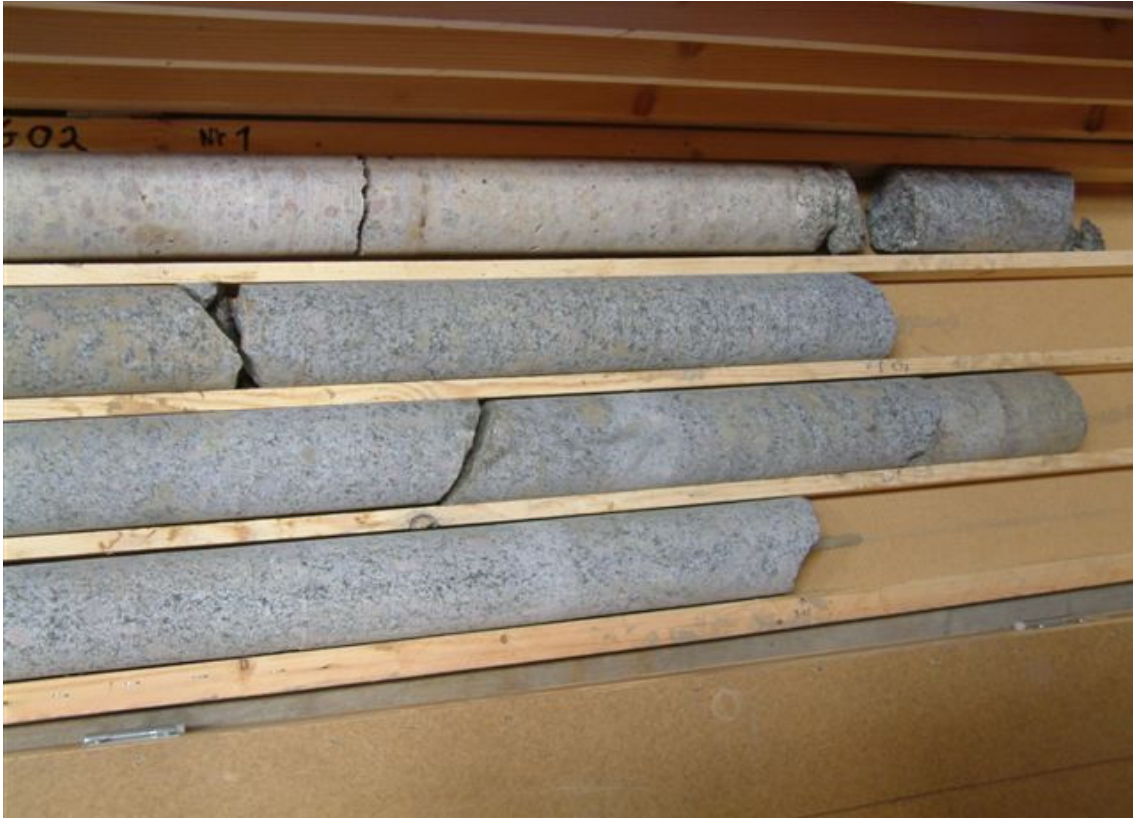
Figure 3-5. Hole KA1621G02. The core representing the lower 2-3 meters of the hole has at least 3 water-bearing fractures.
