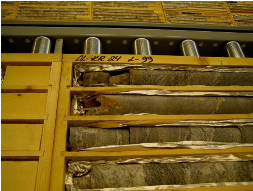
Plate III. Borehole depths 382-384 m (Levels -372 to -374). Upper left part consists of clay/silt material. Photo: R. Pusch.
