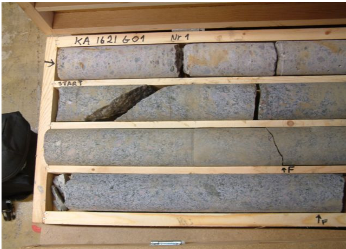
Figure 3-2. Hole KA1621G01. The core representing the uppermost 3 meters of the hole has at least 3 water-bearing fractures.
