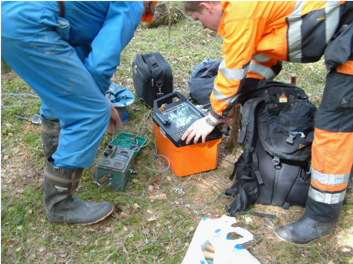
Figure 3-1. The recording instrument, ABEM Terraloc MK6.
