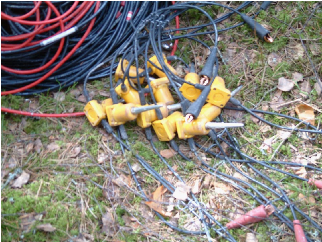
Figur 4-1. Geophones used during the survey.
