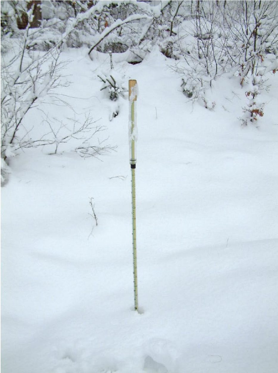
Figure 3-1. Measuring device for registration of depth of frost in the ground at PSM006980.
