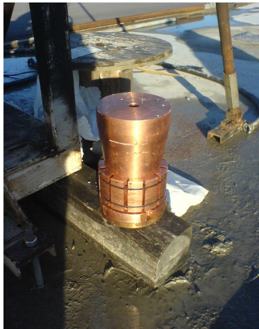
Figure 2-2. The copper “expander” plug. Upper: Function principle. Lower: The copper plug turned upside down below the drill rig before lowering it into the 200 mm hole. The O-rings kept the lamellae in contact with the conical body, which moved them outwards into the recess when applying the pulling force.
