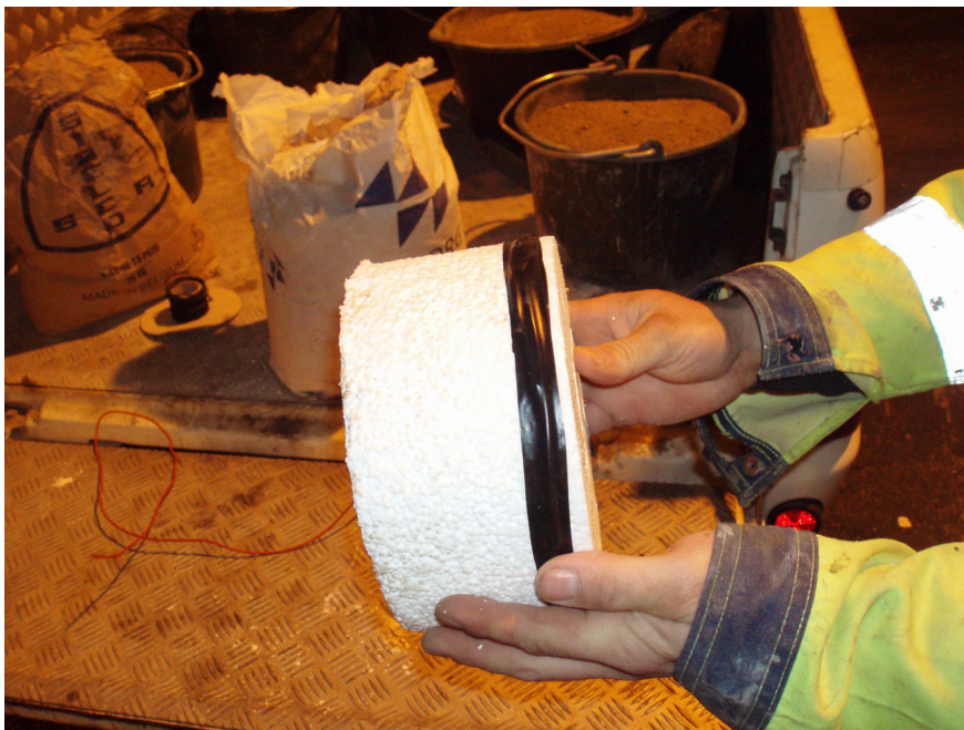
Figure 2-6. Compressible column of porous polystyrene.
