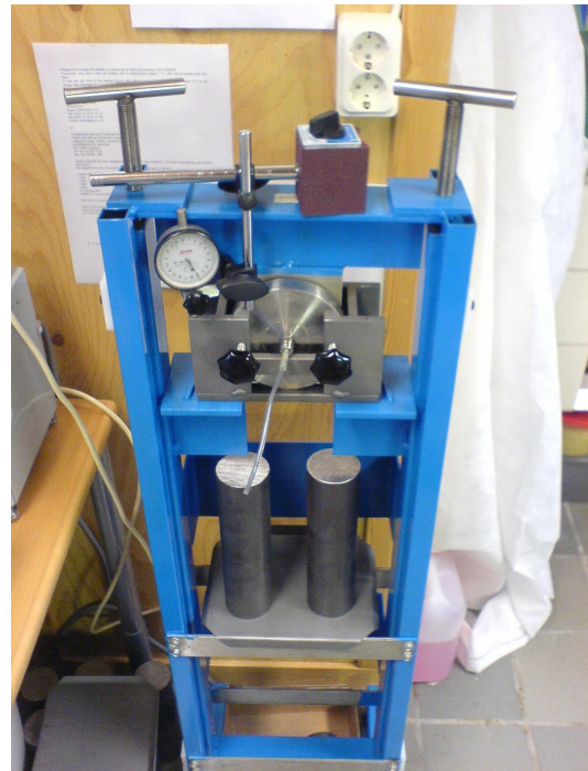
Figure 4. The shear apparatus consists of two cylindrical box halves and a central, movable ring in which the concrete was cast. After 3 weeks the shear box was placed in the apparatus and sheared by applying a load F that acts centrally on the ring.
