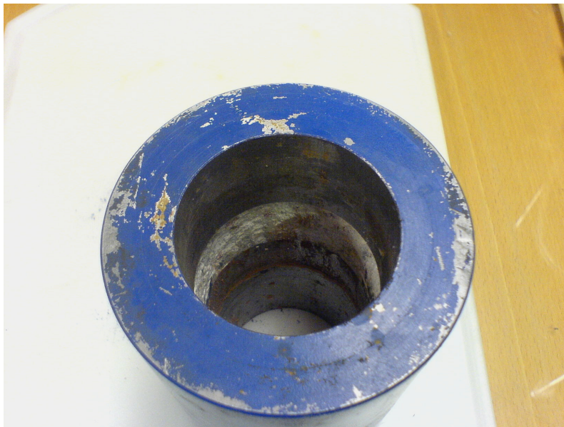
Figure 5. Top view of the form of steel with the sheared concrete with 10 % quartzite fragments seen as a bright band. The broken quartzite fragments that served as reinforcement are seen as white grains in the band.
