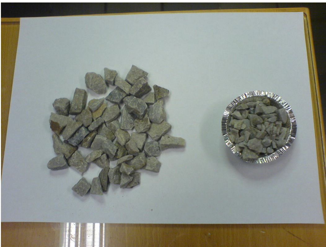
Figure 2. Crushed quartzite as extra aggregate material. Left: Elongated fragments with the long diameter 5-20 mm. Right: Isodiametric fragments with the long diameter 1-10 mm.
