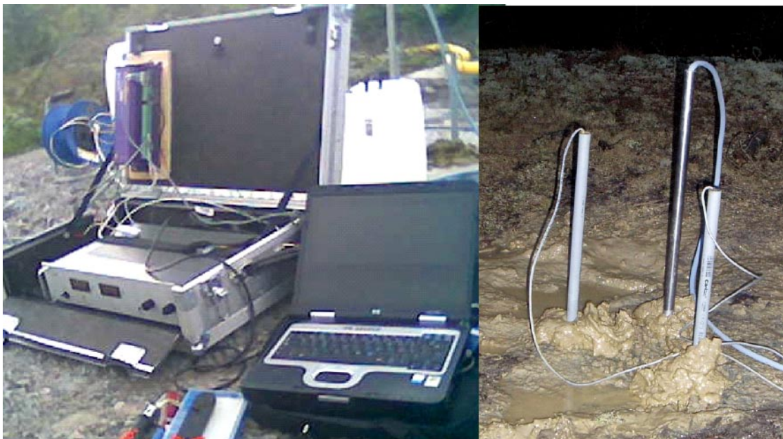
Figure 4-3. Probes for measurements and heating, constant current power supply, data logger and laptop computer for monitoring of data.
