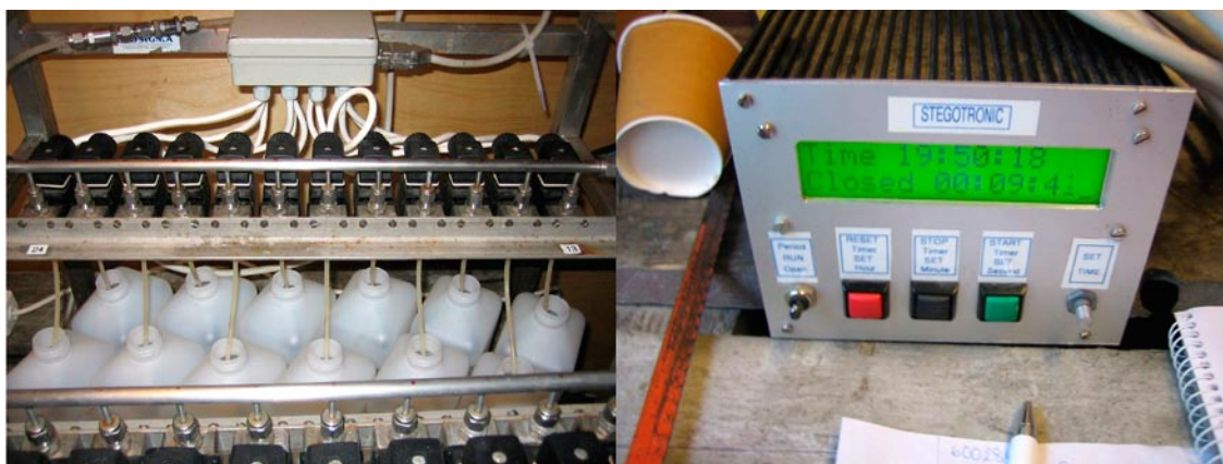
Figure 3-3. The automatic programmable sampler; magnetic valves (left) and control unit (right).
