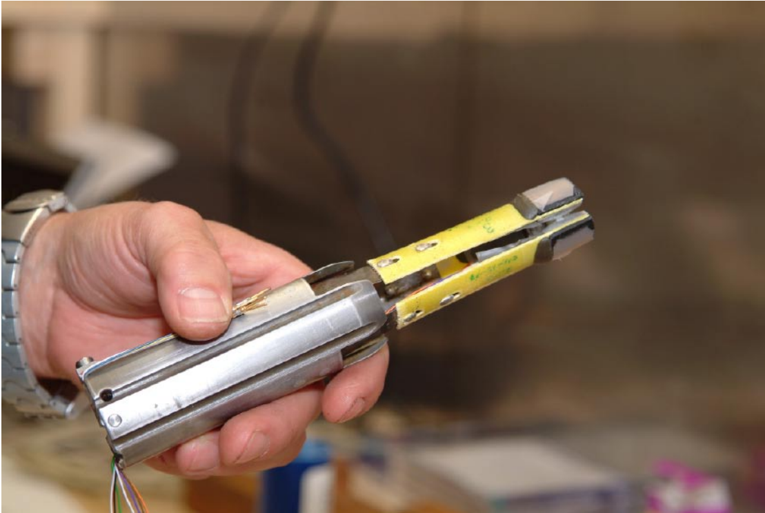
Figure 3-4. A set of strain ganges to be mounted on the Borre probe used for rock stress measurements.
