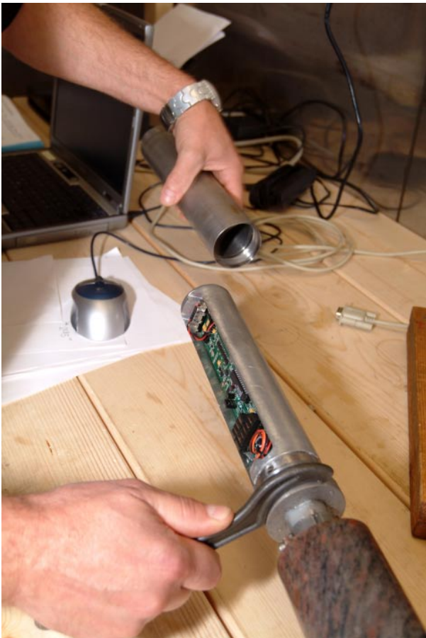
Figure 3-5. Data from the logger unit, part of the Borre probe system, are transferred to the portable computer.
