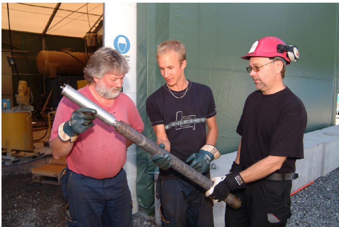
Figure 3-3. Example of an overcored rock sample and the Borre probe from KFM07B.
