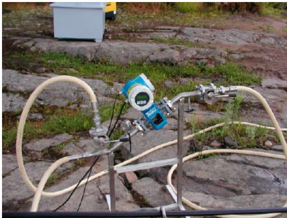
Photo 3. Surface flow meter for measuring total flow rate.
