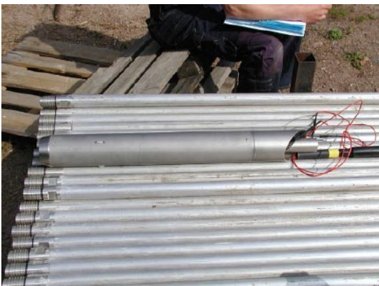
Photo 5. Positioner, bottom end of down-in-hole string.
