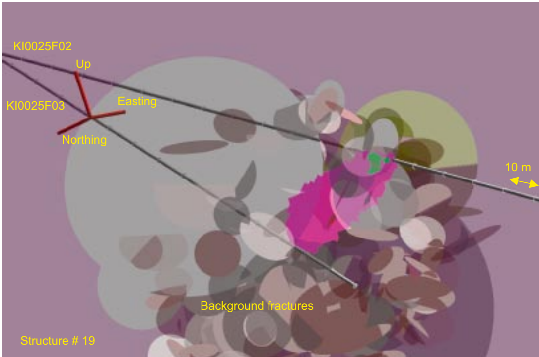
Figure 5-1. BS2B test, injection in Structure #19 – Flow path I. View of the transport path within Structure #19 (“plume” indicated in pink), and of the background fractures (semi-transparent). Result from the ANDRA/Itasca model.
