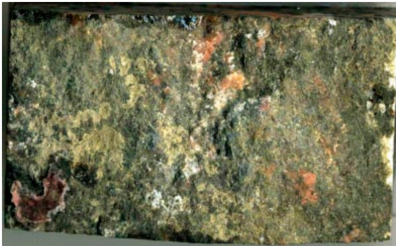
Figure 2-12. Surface of BG1 in borehole KI0025F02 with thin coating of mainly chlorite, calcite, clay minerals and epidote. The length of the base of the photograph is 46 mm.
