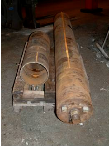
Figure 2-1. 300 mm Core barrels with space for 76 cm and 225 cm core length, respectively
