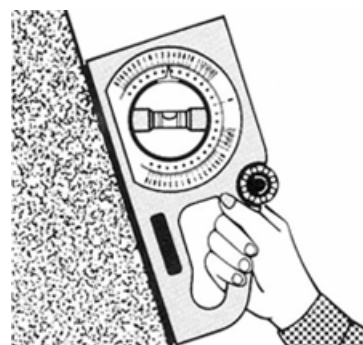
Figure 2-8. Measurement of dip by means of a clinometer with a rotating bubble vial.
