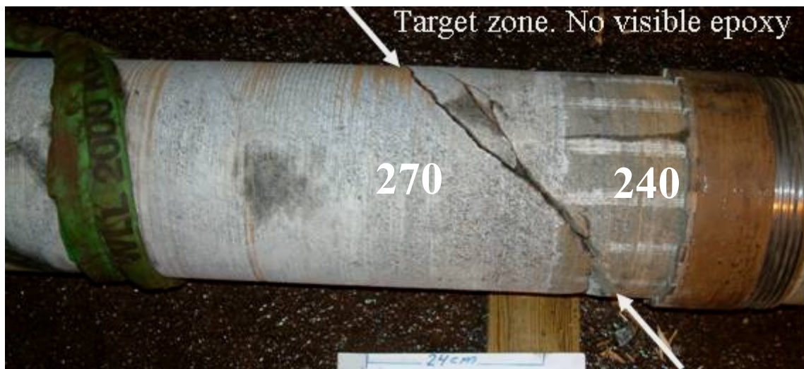
Figure 4-4. KA2169A01. Core recovery with target zone at 250 cm, with no visible epoxy grout. Hidden under the drill bit (far right) are epoxy filled fractures at 210-235 (Figure 4-5).
