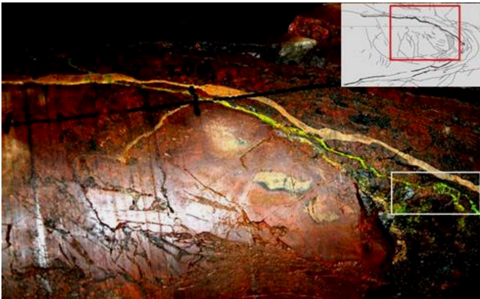
Figure 4-2. KA2549A01. Target zone with diverging fracture zone with epoxy fill, and approximate outline white box of Figure 4-3. Miniature in upper right-hand corner shows approximate coverage of figure in relation to the corresponding envelope drawing in Appendix 1.
