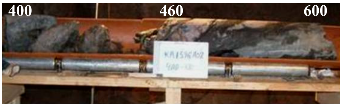
Figure 4-11. KA1596A02. Core recovery with target zone at ca 460 cm.
