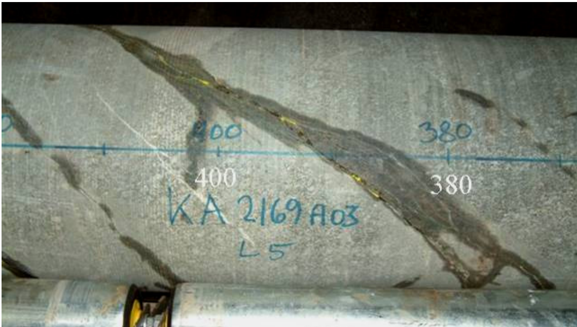
Figure 4-8. KA2169A03. Core recovery with target zone at 390 cm, with plenty of epoxy grout (yellow along the diagonal fracture). The area above the 400 mark is shown in Figure 4-9.
