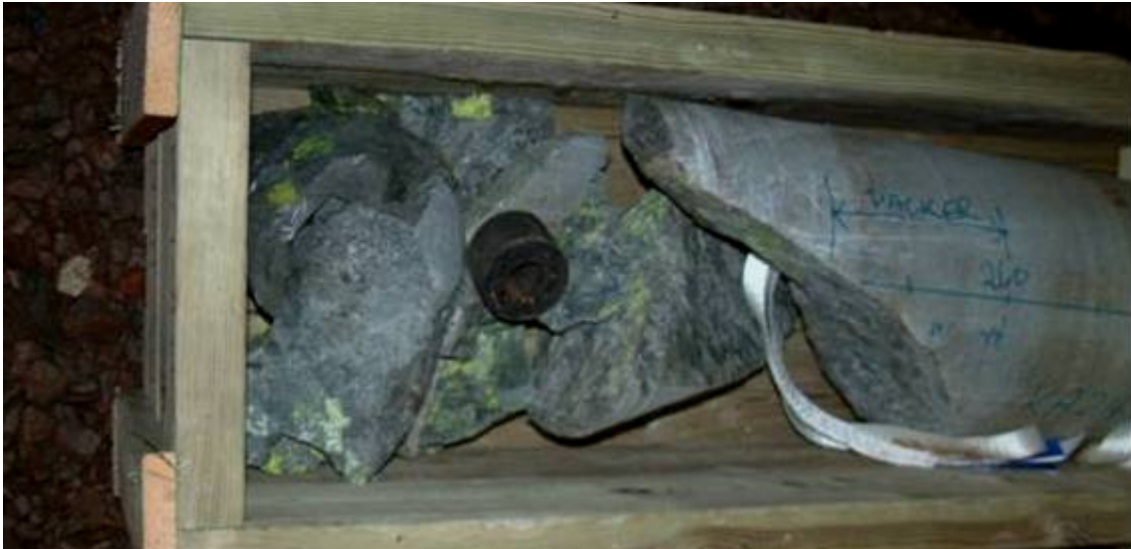
Figure 4-7. KA2169A02. Epoxy patches on fracture surfaces.
