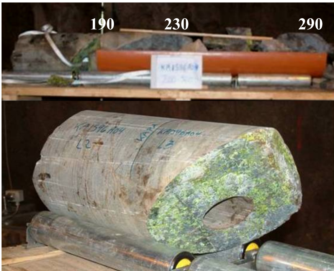
Figure 4-12. KA1596A04. Above: core recovery with epoxy at 190 cm and target zones at 230-320cm. Below: 0°/63° fracture with epoxy at 190 cm.
