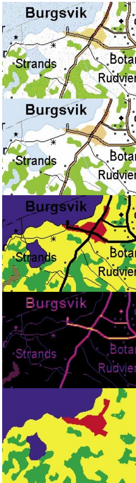
Figure 7-1. Illustration of the principles of the method, where scanned images are treated digitally in order to capture the colours and thereby the land-use without manually vectorising the information. Stefan Ene developed the method.
