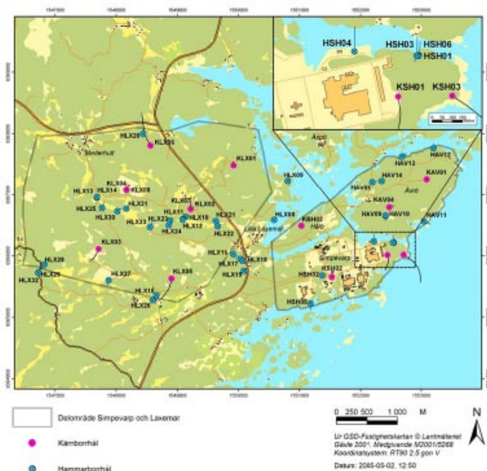
Figure 3-1. Groundwater sampling locations in the Simpevarp area and location of hydrogeochemically prioritised boreholes, KLV01, KLV02, KLV03, KLV04, KLV05, KLV06, KLV07 and KLV08 in the Laxemar subarea. Also indicated are the percussion boreholes (HLX01–33), many of which are included in the Laxemar v.2.1 evaluation. The figure shows the outlines of Laxemar (left hand) and Simpevarp (right hand) subareas.
