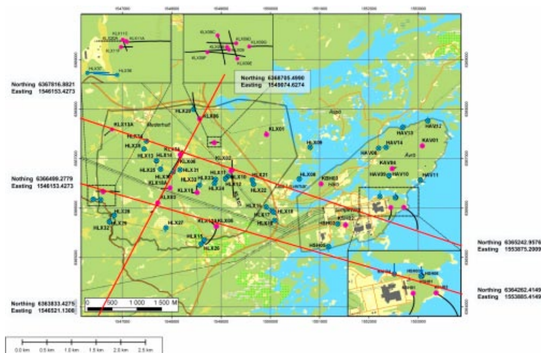
Figure 2-13. Plan view of the traces of the 3 selected cross sections to extract computed results from the hydrogeological models.
