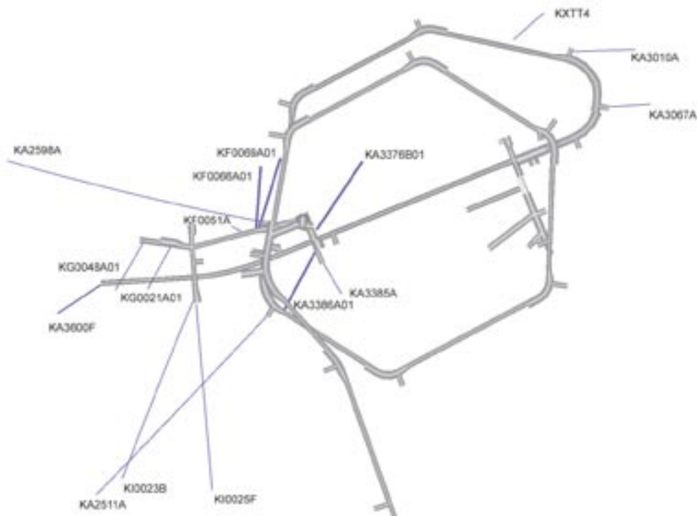
Figure 2-2. Core borehole KA3376B01 and core boreholes where pressure is monitored using HMS (not monitored for KF0066A01).
