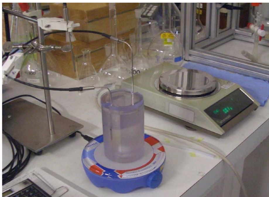
Figure 3-3. Calorimeter with two temperature sensors on magnetic stirrer.
