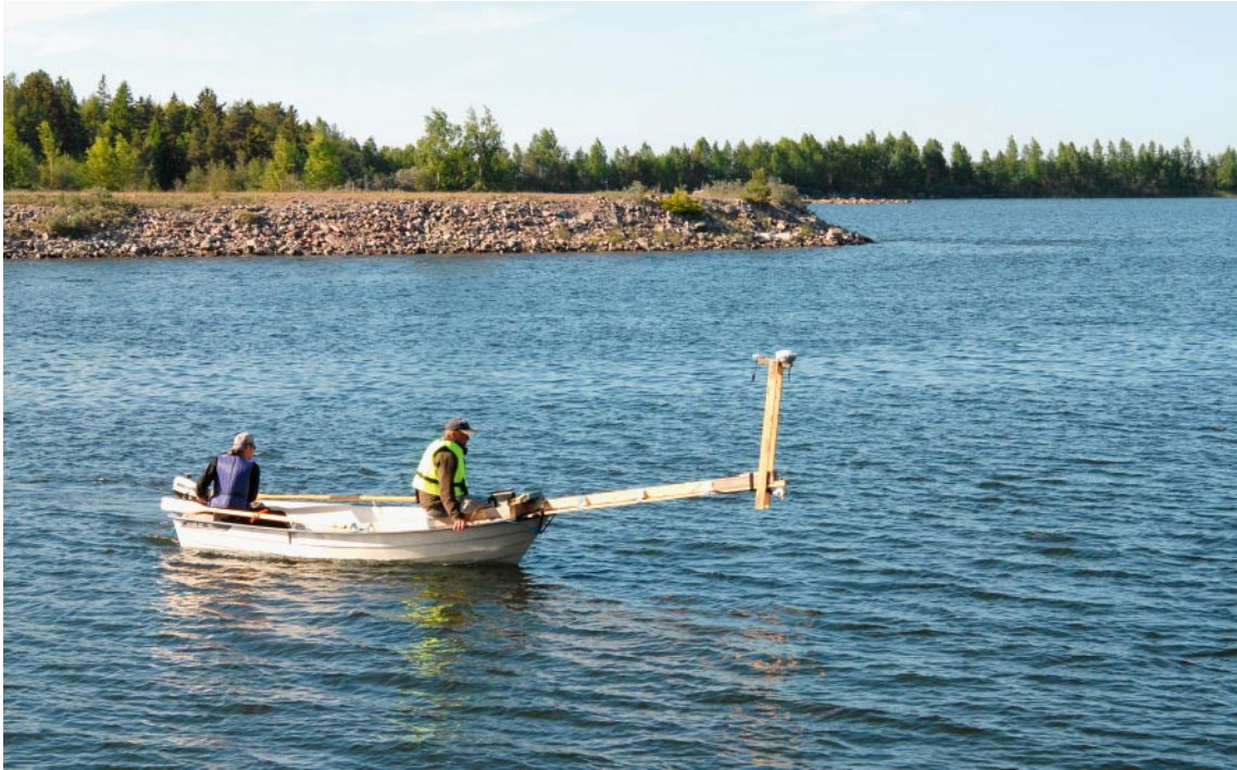
Figure 3-1. Magnetic marine survey on Asphällsfjärden using a small boat. The magnetic sensor is placed on a wooden frame in front of the boat. The RTK-GPS-antenna is mounted approximately one metre above the magnetometer. Photo: Alf Sevastik.
