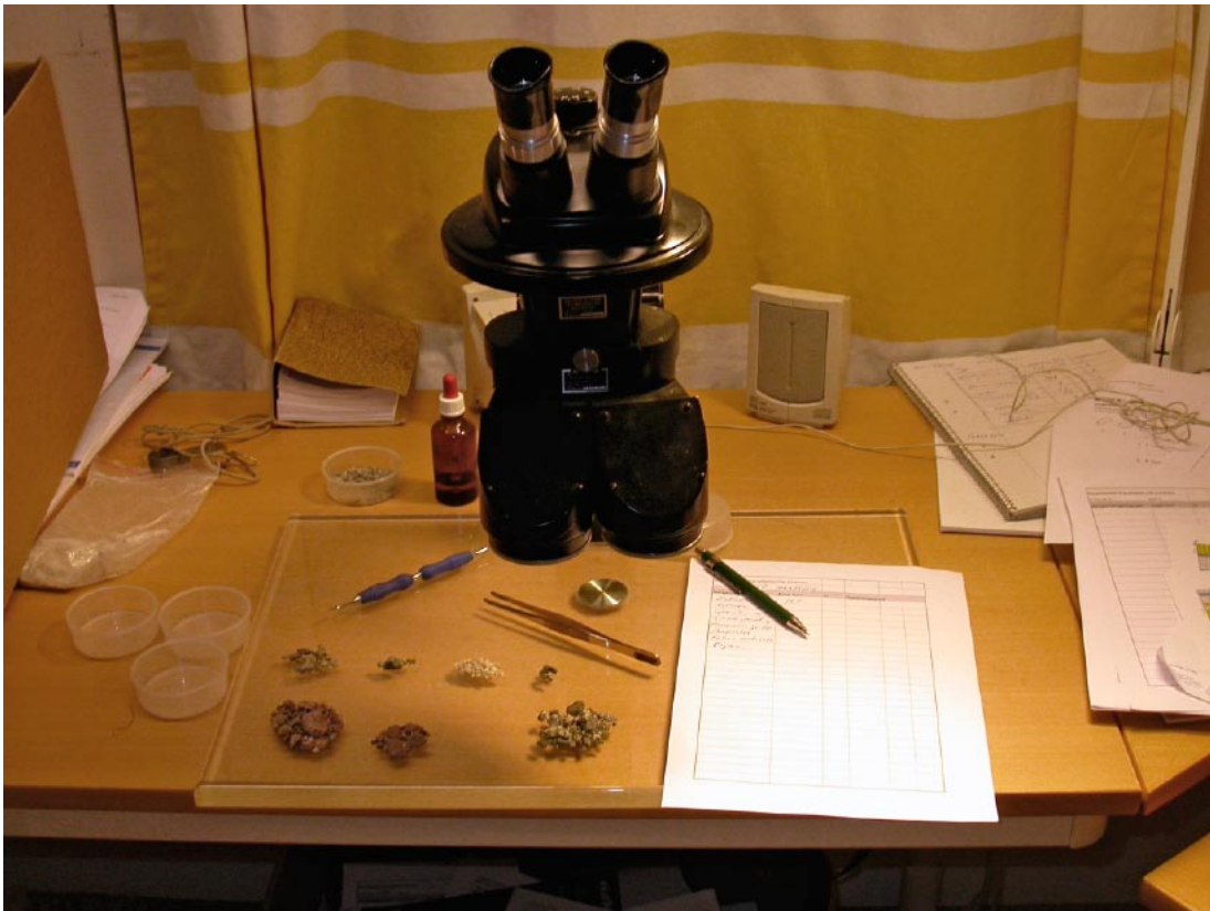
Figure 3-1. Laboratory set-up for petrographic analysis of washed gravel samples.
