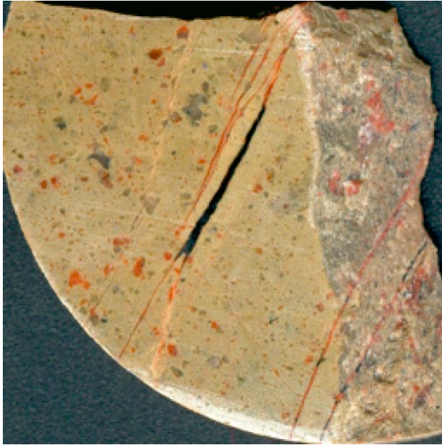
Figure 5-15. K-feldspar (red), quartz and chlorite (black) in fractures that cut through mylonite/cataclasite. Photograph from a sawed piece of the sample.
