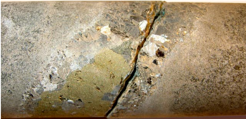
Figure 5-28. Photograph of the drill core showing a fracture sealed with muscovite, pyrite, quartz and calcite (not visible in the photograph).
