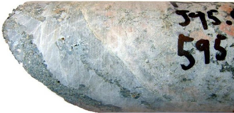
Figure 5-32. Photograph of the drill core showing a fracture sealed with mainly muscovite, quartz and fluorite.
