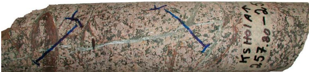
Figure 5-3. Sample KSH01A: 256.90–257.10 m. Sealed fractures (generation 6), filled with calcite, adularia, Mg-chlorite, Fe-chlorite and pyrite etc. are cutting through brown-coloured cataclasite.
