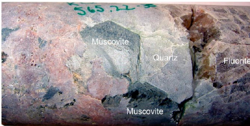
Figure 5-30. Photograph of the drill core showing a fracture sealed with muscovite, quartz and fluorite.
