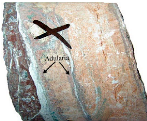
Figure 5-10. Cataclasite (generation 2, red-brown coloured, left) is cut by calcite-filled fractures (generation 3, white colour). The latest formed fractures are filled with adularia (generation 6) and laumontite, (orange colour).
