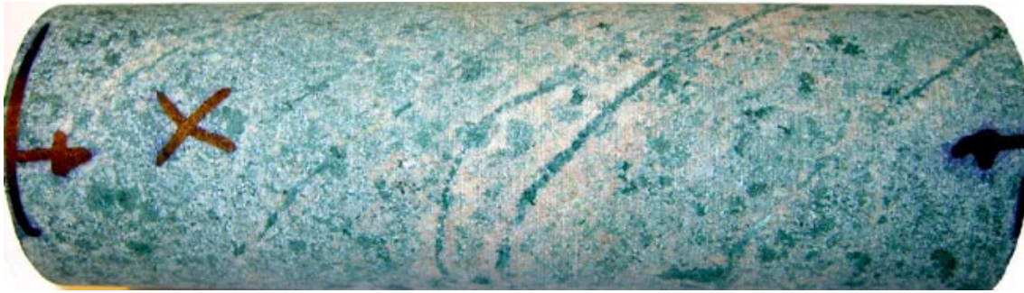
Figure 5-34. Photograph of the drill core showing fractures sealed with mainly hornblende, calcite, K-feldspar and chlorite.
