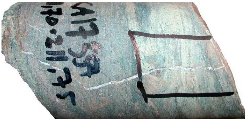
Figure 5-1. KA1755A: 211.70–211.75 m. Mylonite (generation 1), cut by a fracture filled with calcite (white), fluorite and hematite.
