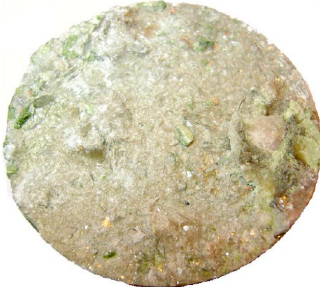
Figure 5-24. Photograph of the fracture surface covered with apophyllite.
