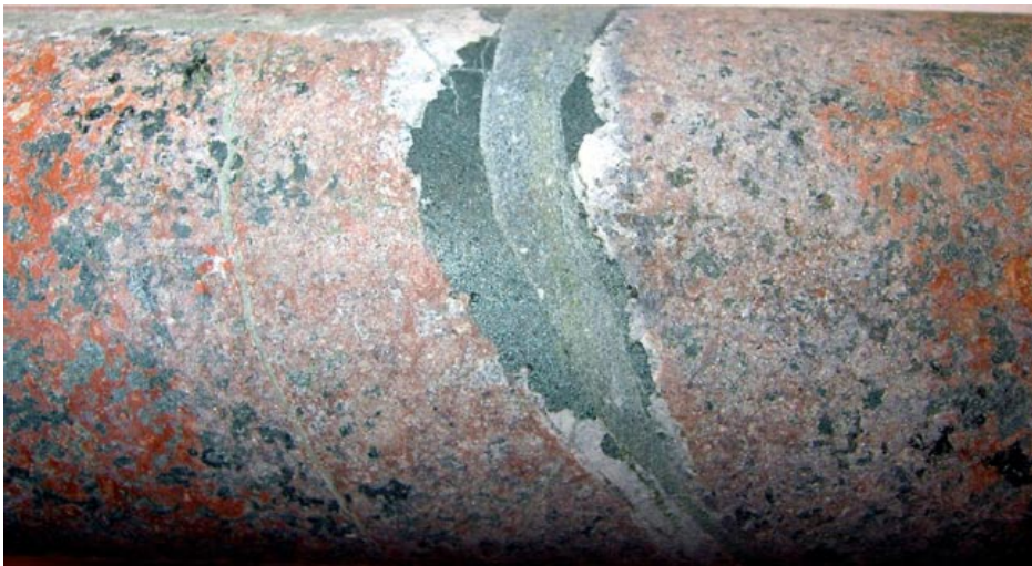
Figure 5-21. Photograph of the drill core showing a fracture sealed with calcite, quartz and chlorite and subsequently prehnite. The red-stained wall rock is bleached close to the fracture, due to a high amount of muscovite in the altered plagioclase.
