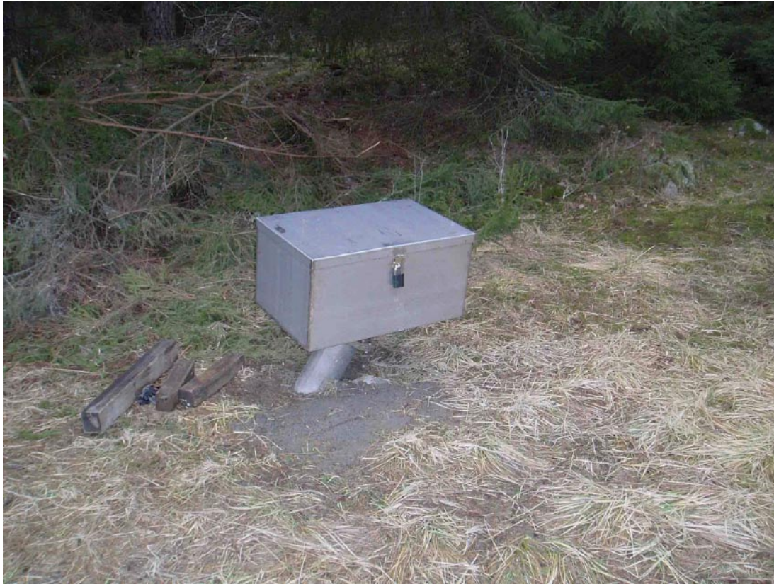
Figure 4-7. Steel cap fitted on casing in HLX42.
