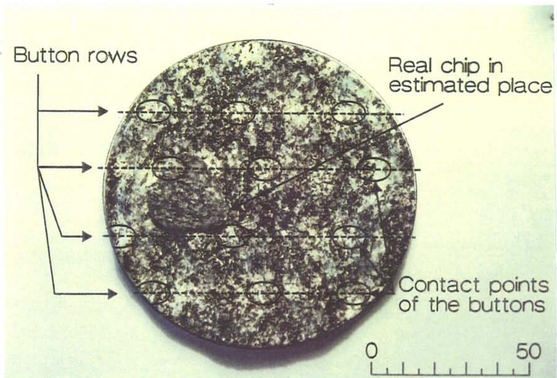
Figure 6.4-24. Photographs of a sample taken from the bottom of a large hole. The location of the button rows, contact points and a chip are shown. As seen, the positions of contact points form an irregular pattern with varying spacing between successive contact points.
