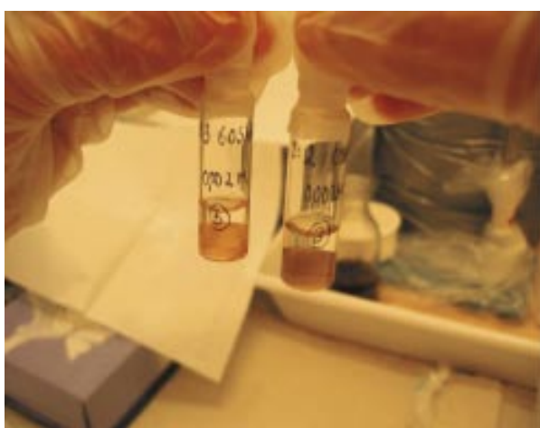
Figure 3-9. Samples containing different ratios of calixarene and COSAN. Ratio 1:3 to the left and ratio 1:2 to the right.
