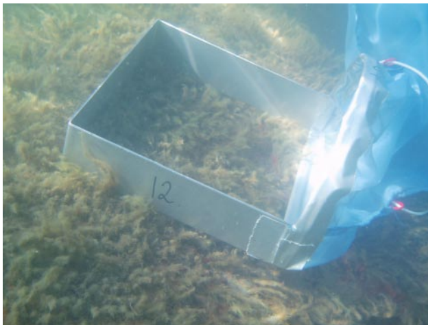
Figure 3-2. A bag attached to one open side of an ID-marked steel frame was used to collect the entire content within the in situ chambers.
