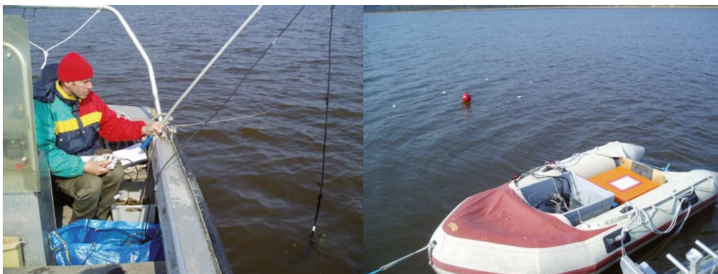
Figure 4-4. A stick was used during PAR measurements to prevent shadows from the boat influencing the readings (left). For the same reason the rubber boat used for the logging devices were anchored away from the in situ measurements (right).
