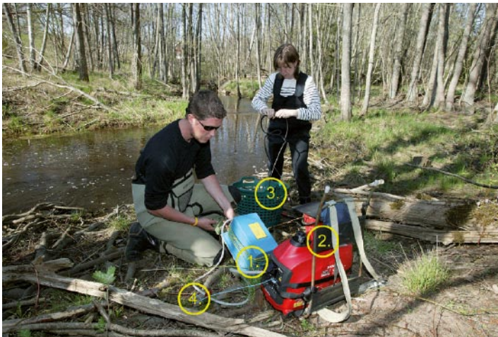
Figure 3-1. Electrofishing equipment. 1:Transformer, 2: Power unit, 3: Cable connecting transformer and anode, 4: Ground cable.
