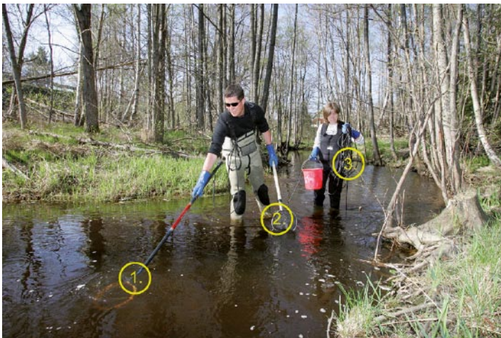
Figure 3-2. Electrofishing equipment. 1: Electrofishing pole with anode, 2: Net, 3: Cable connecting transformer and anode (+).
