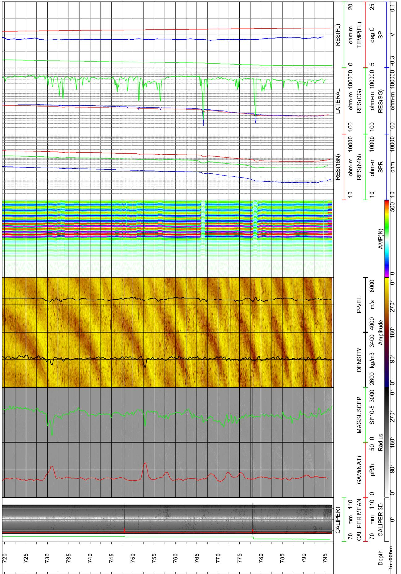
**Borehole KLX28A. Drawing no. 2.1. Borehole logs**
