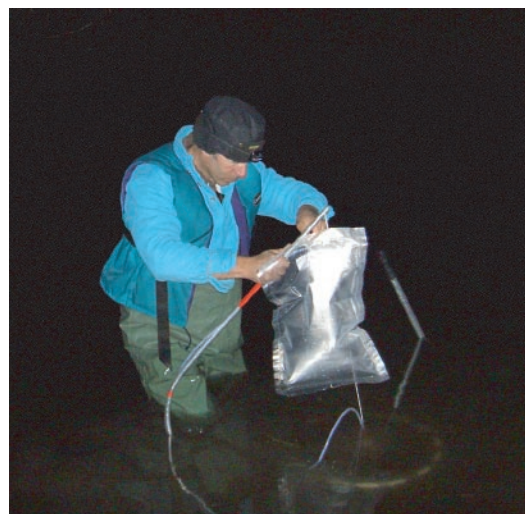
Figure 2-2. Sampling of gas in sediments, starting (left) and finishing (right).
